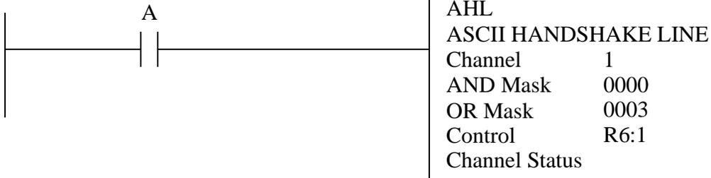
**Description:** This instruction will check the serial interface using the DTR and RTS send bits. Bit 0 is DTR and bit 1 is the RTS. If a bit is set in the AND mask the bits will be turned off, otherwise they will be left alone. If a bit is set in the OR word a bit will be turned on, otherwise they will be left alone. In this example the DTR and RTS bits will be turned on for channel 1.
