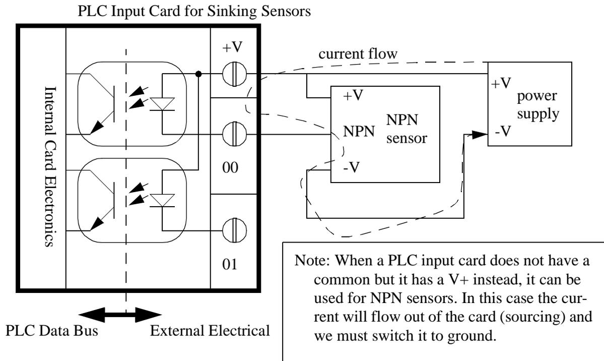
**ASIDE:** This card is shown with 2 optocouplers (one for each output). Inside these devices there is an LED and a phototransistor, but no electrical connection. These devices are used to isolate two different electrical systems. In this case they protect the 5V digital levels of the PLC computer from the various external voltages and currents.
