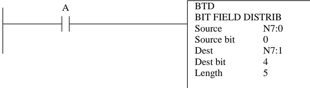
Description: This function will copy the bits starting at N7:0/0 to N7:1/4 for a length of 5 bits.
