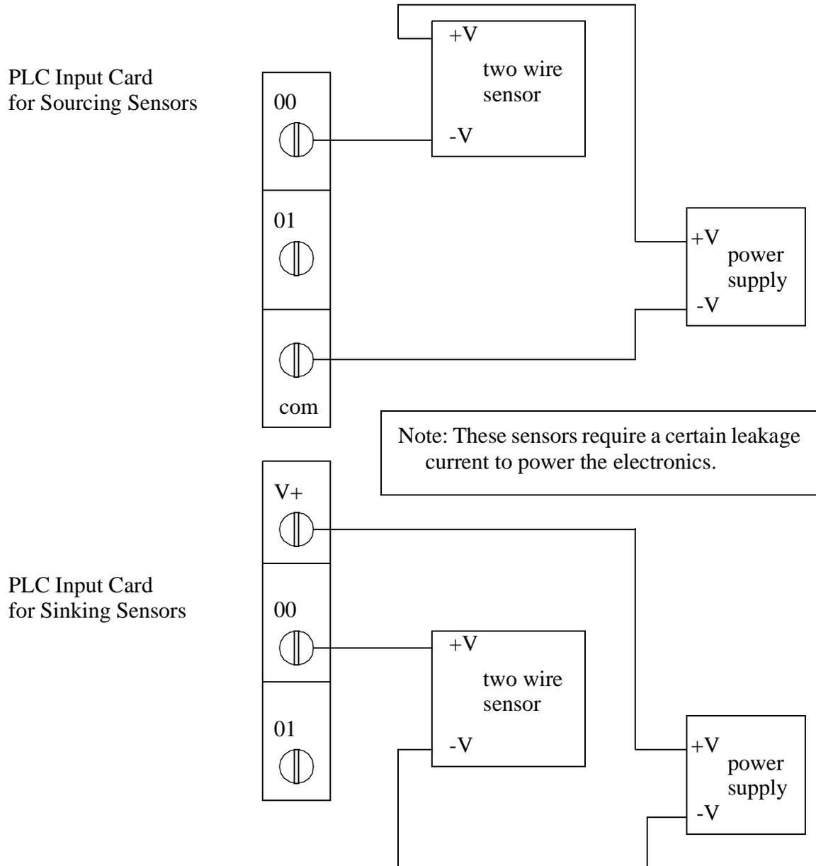
*Figure 4.8* Two Wire Sensors
