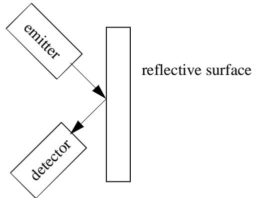
*Figure 4.18* Detecting Reflecting Parts
