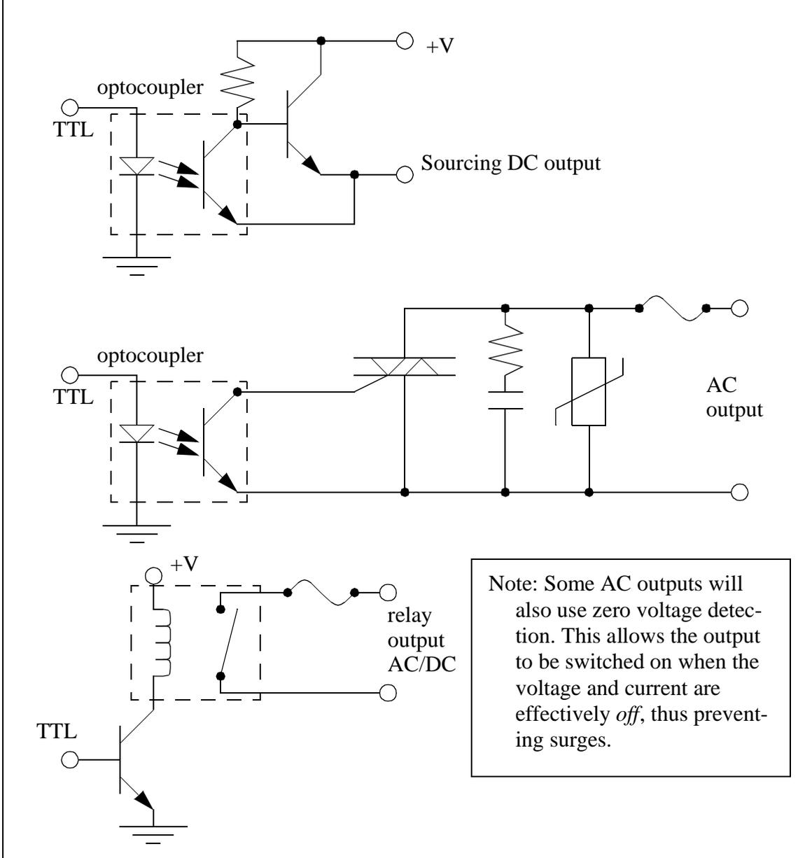
Note: Some AC outputs will also use zero voltage detection. This allows the output to be switched on when the voltage and current are effectively *off*, thus preventing surges.
