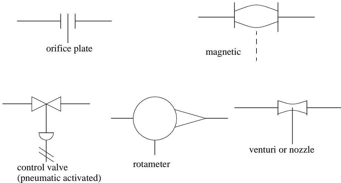
Figure 32.4 Sensor and Actuator Symbols and Types
