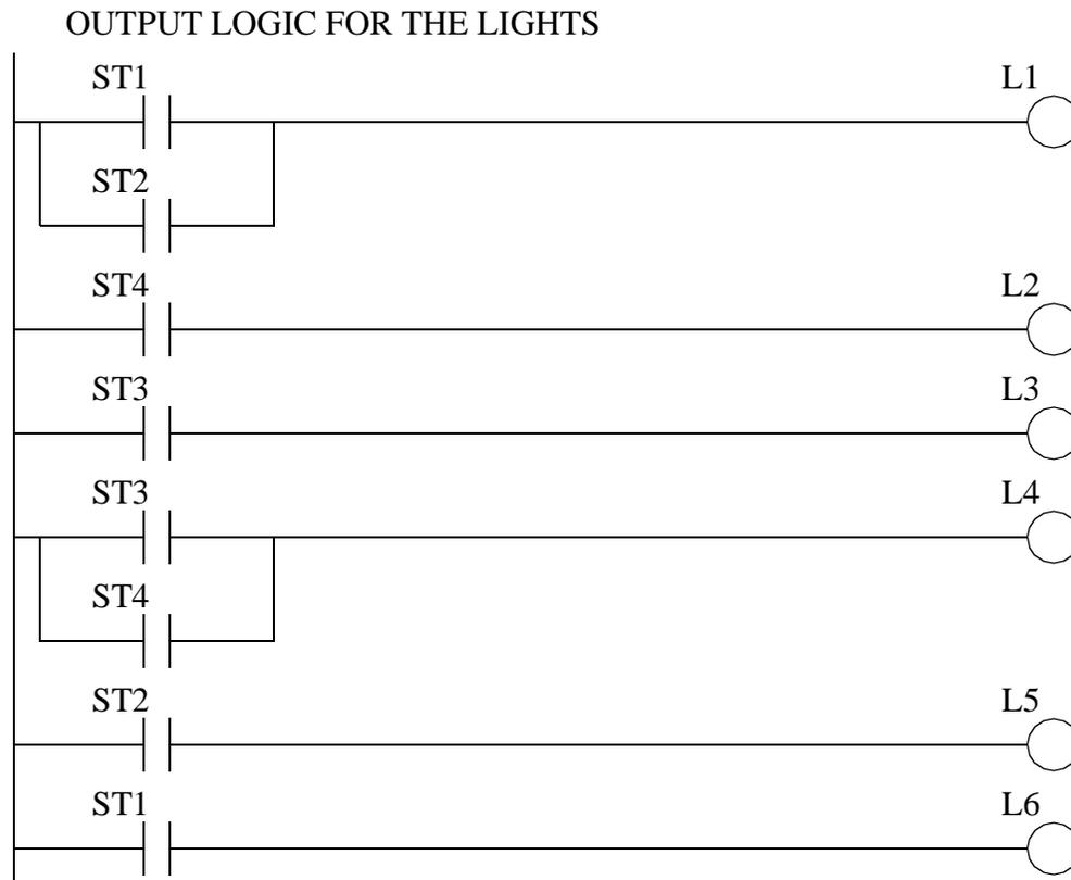
*Figure 12.23* Ladder Logic for the State Equations
