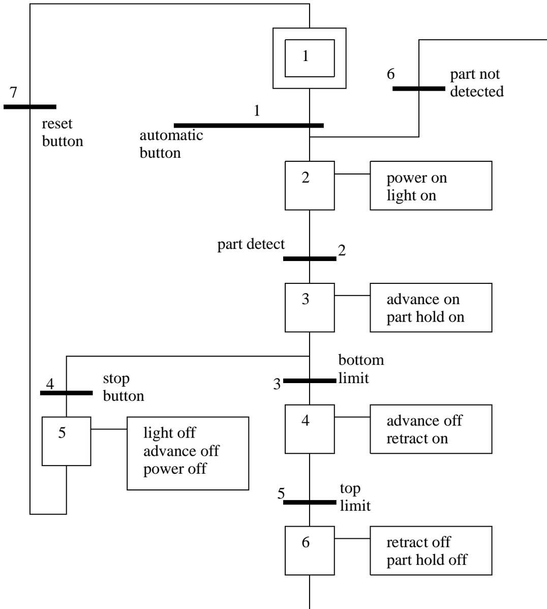
Figure 20.4 SFC for Controlling a Stamping Press
