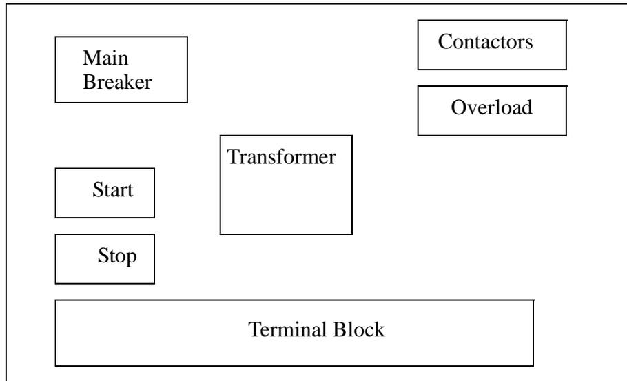
*Figure 31.2* A Physical Layout for the Control Cabinet
