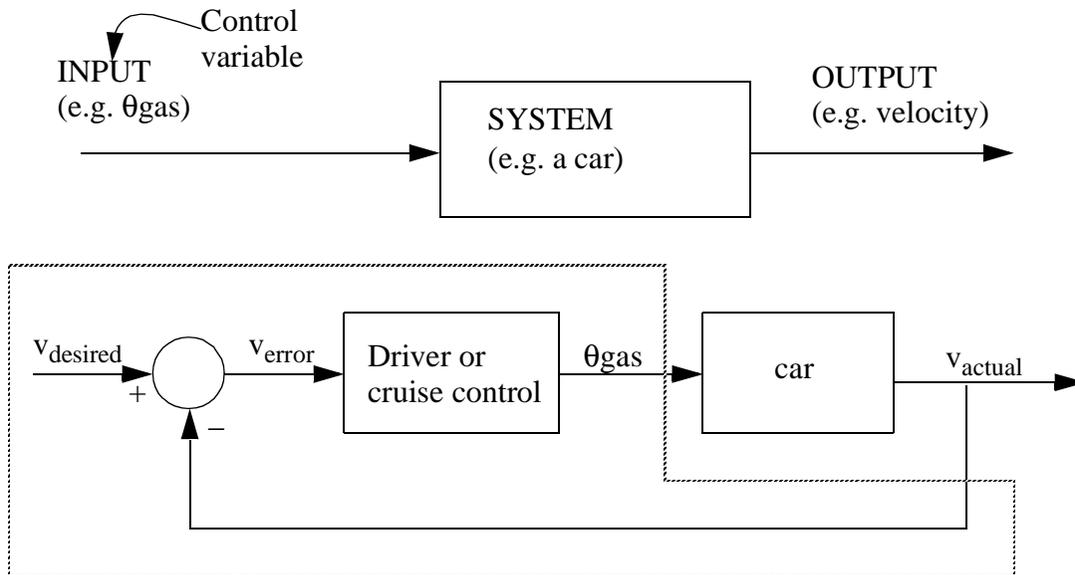
Figure 25.6 Addition of a Control System to a Car
