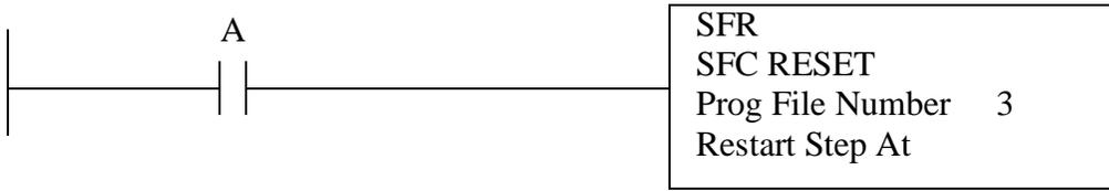
Description: This function will reset a SFC. In this example when 'A' goes true the SFC main program stored in program file 3 will be examined. All sub programs will be examined, and then the SFC will be reset to the initial position.
