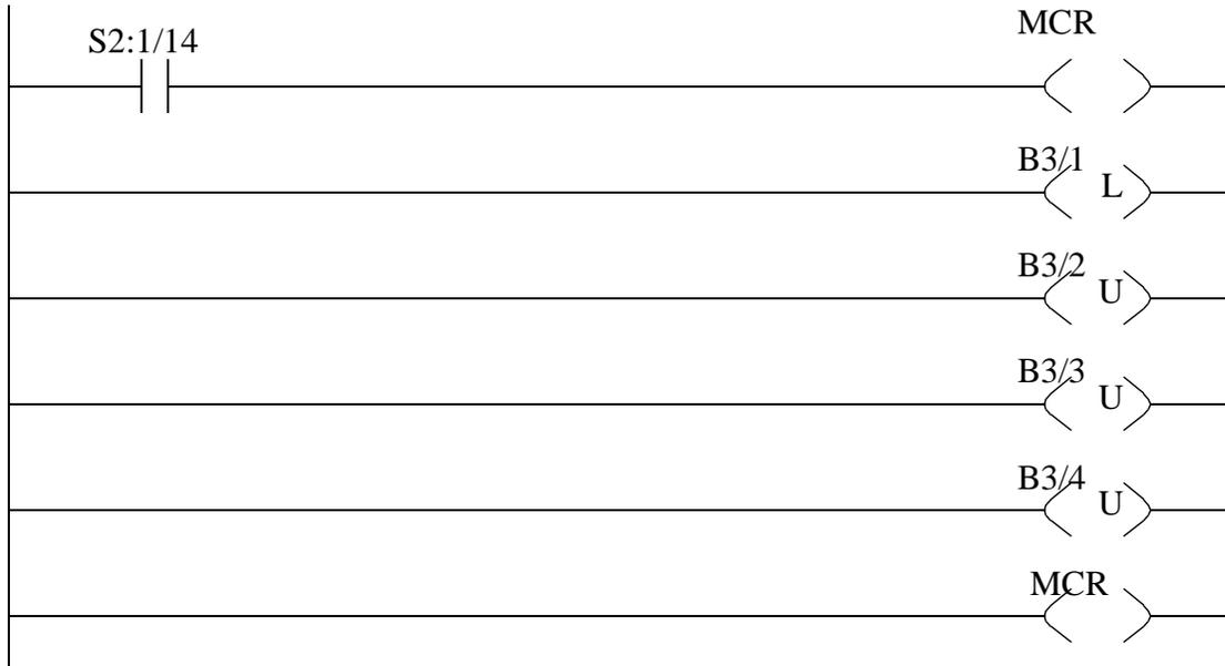
Figure 12.10 Ladder Logic to Initialize Traffic Light Controller
