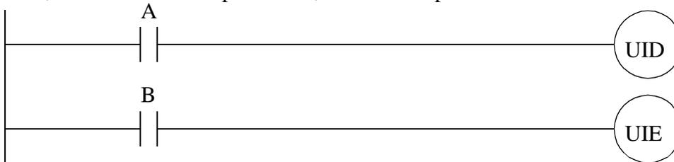
Description: This instruction is used to turn off interrupts. If 'A' is true, then the following ladder logic will be run without interrupts. If 'B' is true the interrupts will be reenabled. These instructions will only be of concern when using user programmed interrupt functions. These are normally only used when a critical process may be completed within a given time, or when the ladder logic between the UID and UIE conflicts with one of the interrupt programs.
