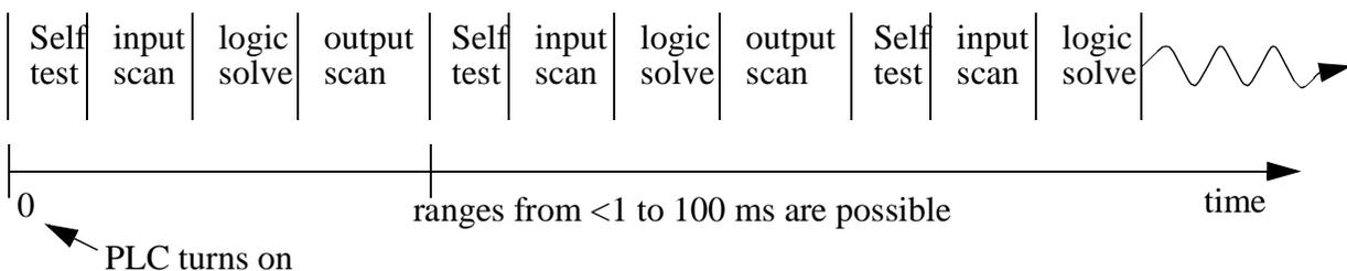
**SELF TEST** - Checks to see if all cards error free, reset watch-dog timer, etc. (A watchdog timer will cause an error, and shut down the PLC if not reset within a short period of time - this would indicate that the ladder logic is not being scanned normally).
