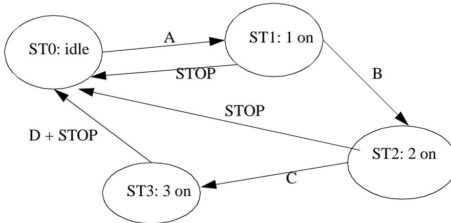
4. Convert the following state diagram to ladder logic using the delayed update method.
