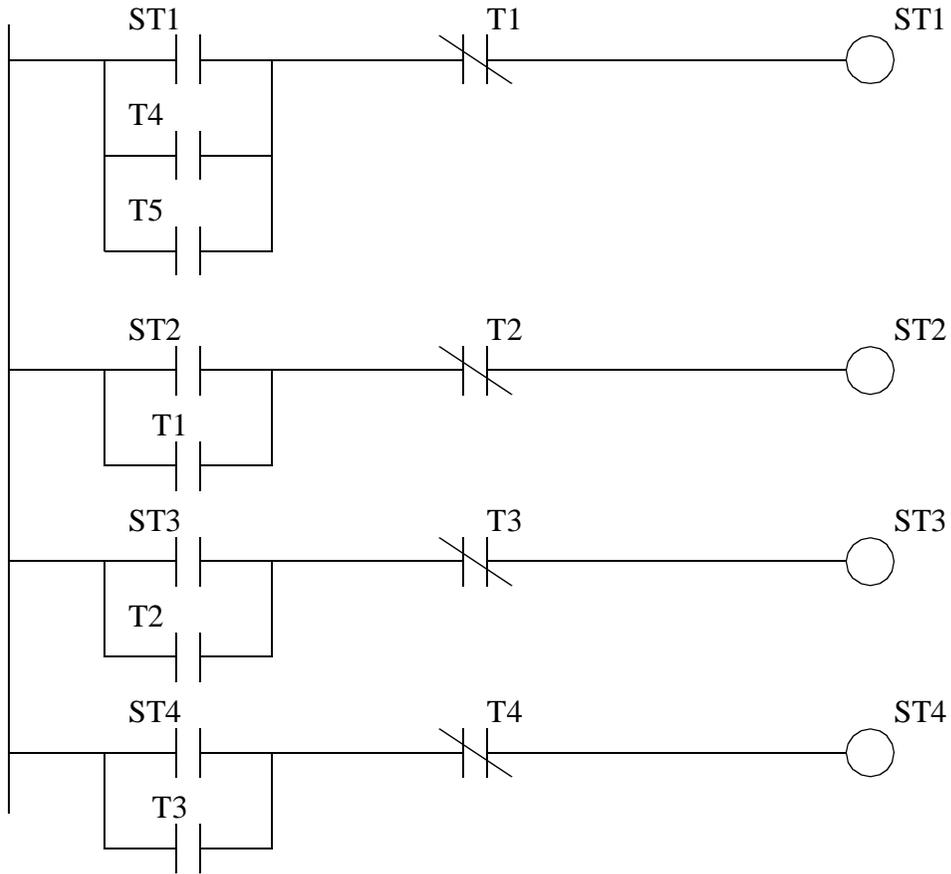
Figure 12.29 Ladder Logic for the State-Transition Equations
