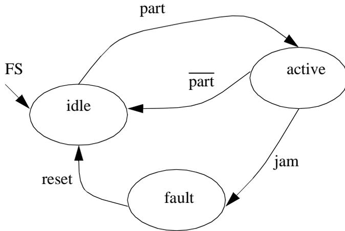
5. Use equations to develop ladder logic for the state diagram below using the delayed update method. Be sure to deal with the priority problems.
