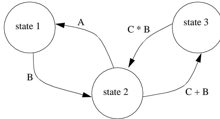
5. Convert the following state diagram to logic using equations.
