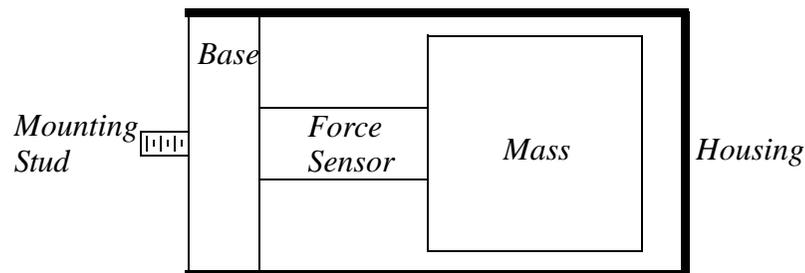
*Figure 23.12* A Cross Section of an Accelerometer
