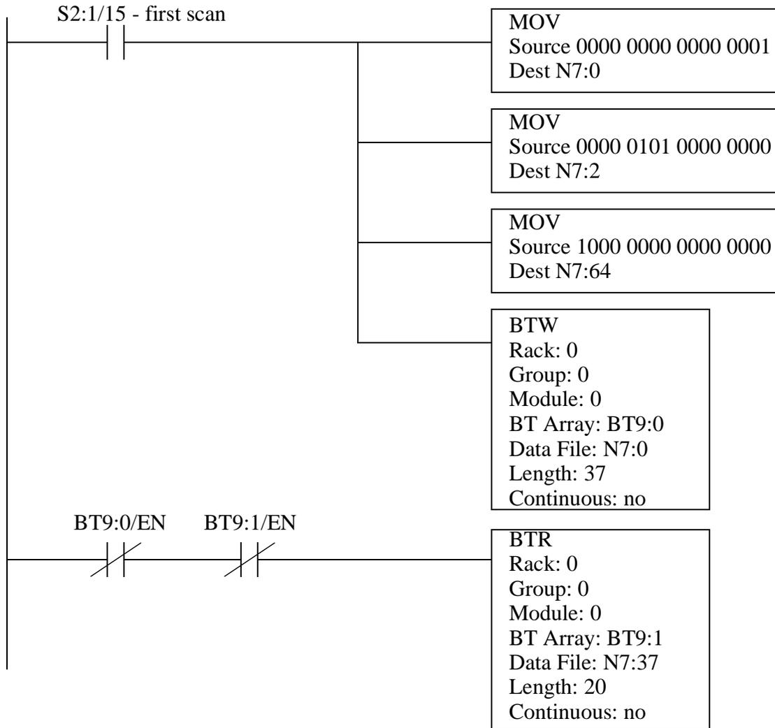
Figure 25.20 A Water Tank Level Control Program
