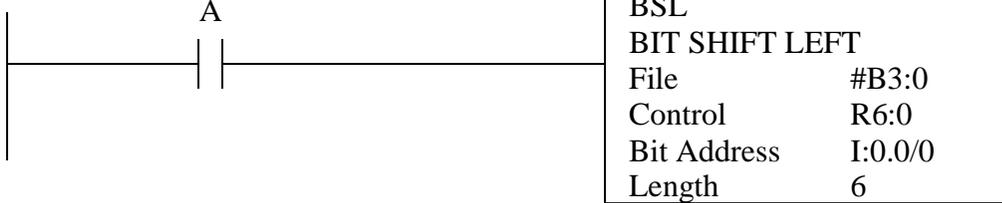
**Description:** These functions will shift bits through left or right through a string of bits starting at #B3:0 with a length of 6 in the example above. As the bits shift the bit shifted out will be put in the UL bit. A new bit will be shifted into the vacant spot from the Bit Address. When the bits are shifted they are moved in the memory locations starting at file #B3:0.
