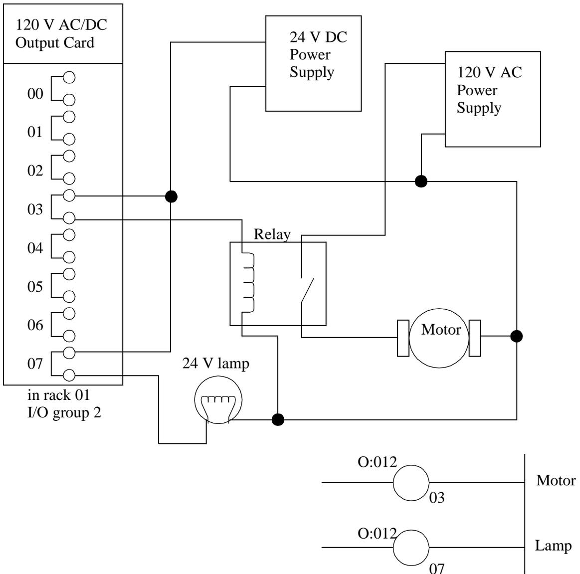
Figure 3.7 An Example of a Relay Output Card
