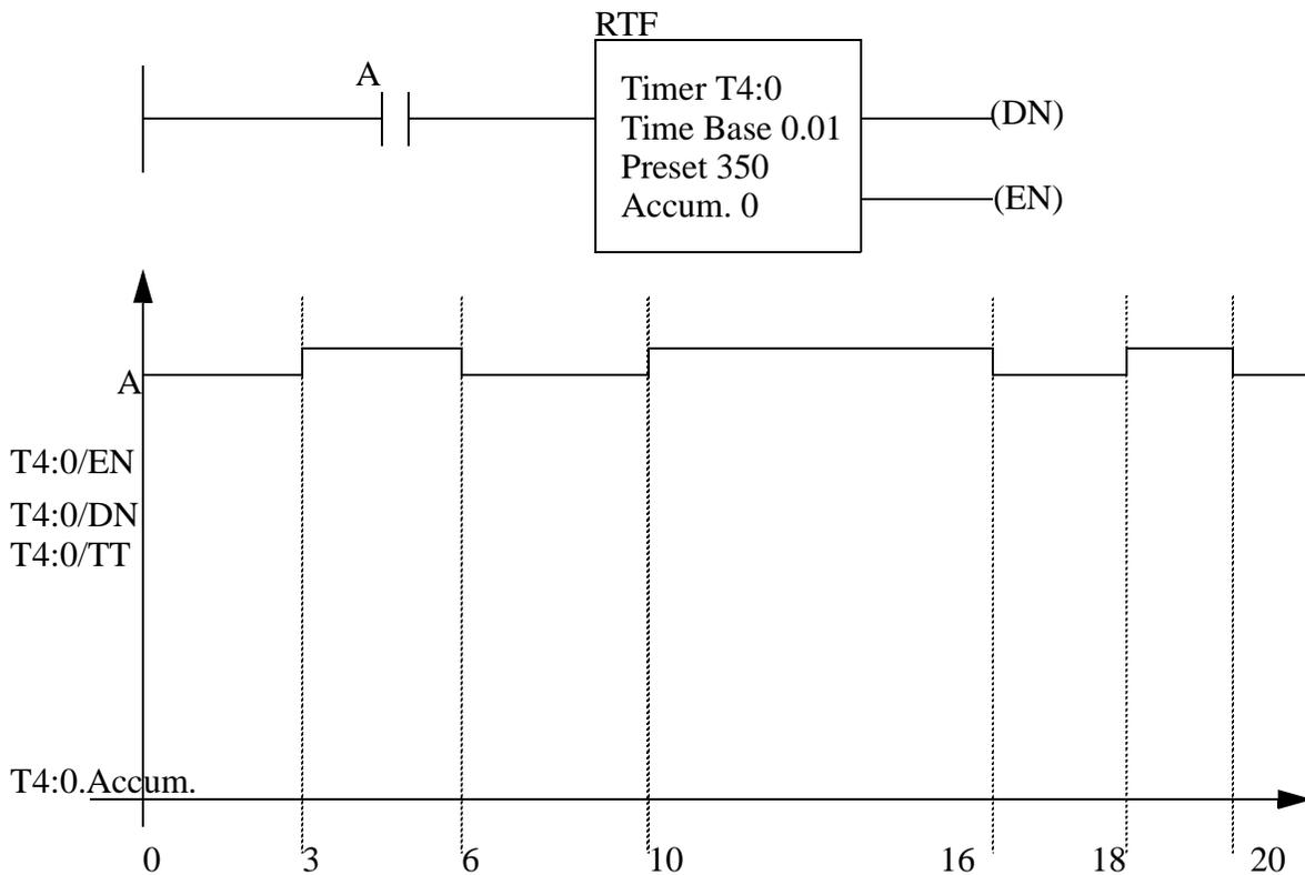
8. Complete the timing diagrams for the two timers below.
