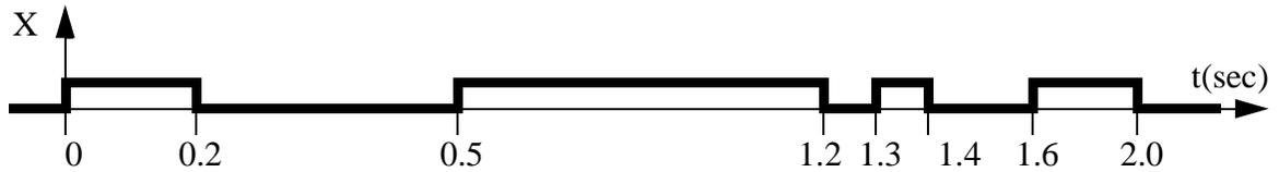
2. Use the timing diagram below to design ladder logic. The sequence should start when input *X* turns on. *X* may only be on momentarily, but the sequence should continue to execute until it ends at 26 seconds.
