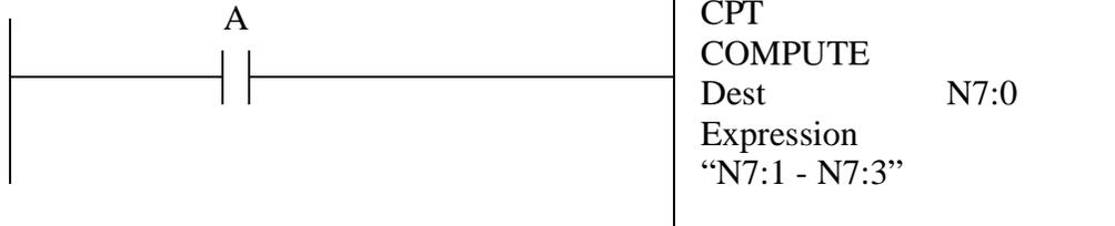
**Description:** This expression allows free-form entry of equations. A maximum of 80 characters is permitted. Operations allowed include +, -, | (divide), \*, FRD, BCD, SQR, AND, OR, NOT, XOR, \*\* (x\*\*y = x to power y), RAD, DEG, LOG, LN, SIN, COS, TAN, ASN, ACS, ATN
