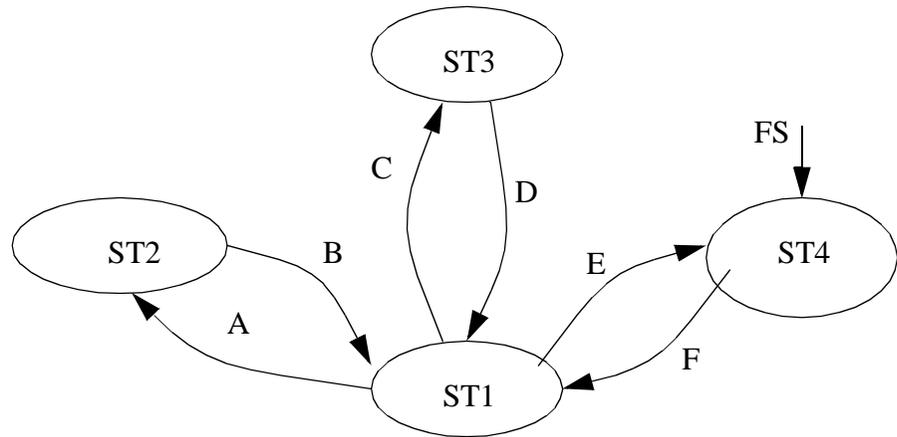
4. Given the following state diagram, use equations to implement ladder logic.
