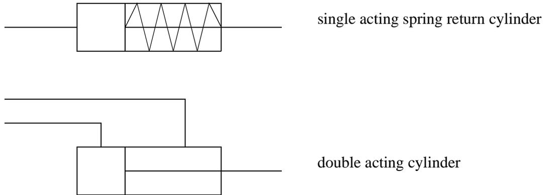
*Figure 5.5* Schematic Symbols for Cylinders
