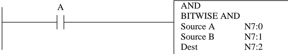
**Description:** These functions do basic boolean operations to the numbers in locations A and B. The results of the operation are stored in Dest. These calculations will be performed whenever the input is true. The functions are,
