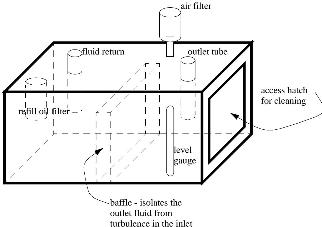
*Figure 5.6*     A Hydraulic Fluid Reservoir
