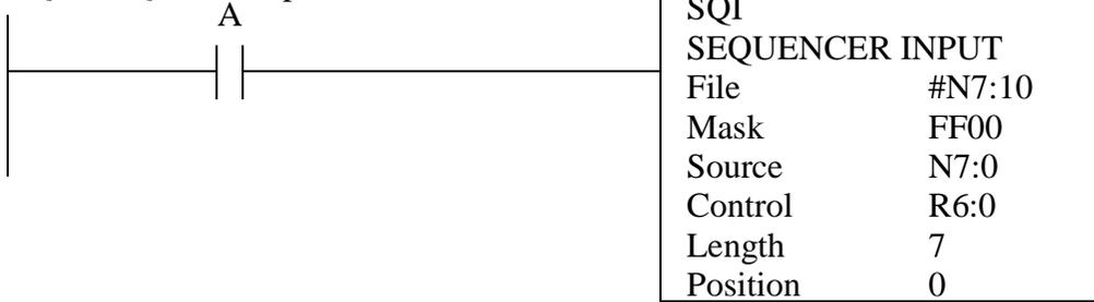
**Description:** This will compare a source value to a set of values in a sequencer table. In this example the 8 most significant bits of 'N7:0' will be loaded each time 'A' goes from false to true. The sequencer will load words from 'N7:10' to 'N7:17'.
