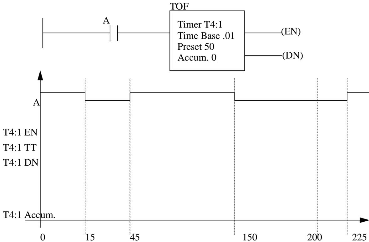
9. Given the following timing diagram, draw the done bits for all four fundamental timer types. Assume all start with an accumulated value of zero, and have a preset of 1.5 seconds.
