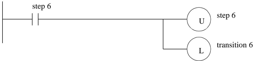
*Figure 20.9* SFC Implemented in Ladder Logic
