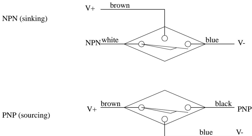
Figure 4.9 Sourcing and Sinking Schematic Symbols
