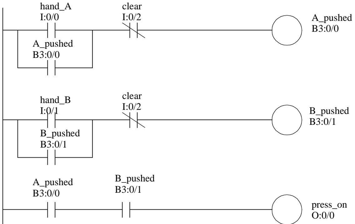
Figure 9.20 An example using bit memory
