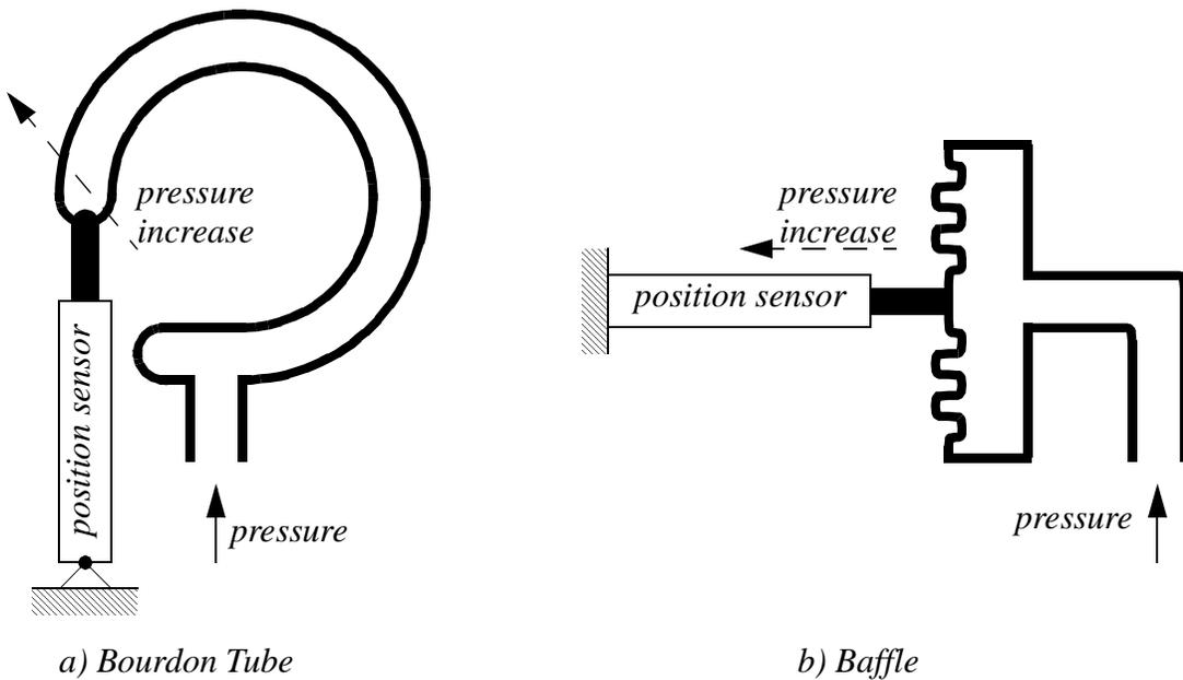
Figure 23.22 Pressure Transducers
