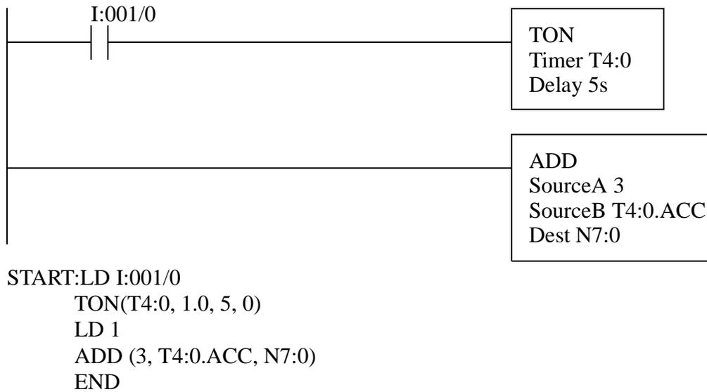
*Figure 18.6* A Complex Ladder Rung and Equivalent IL
