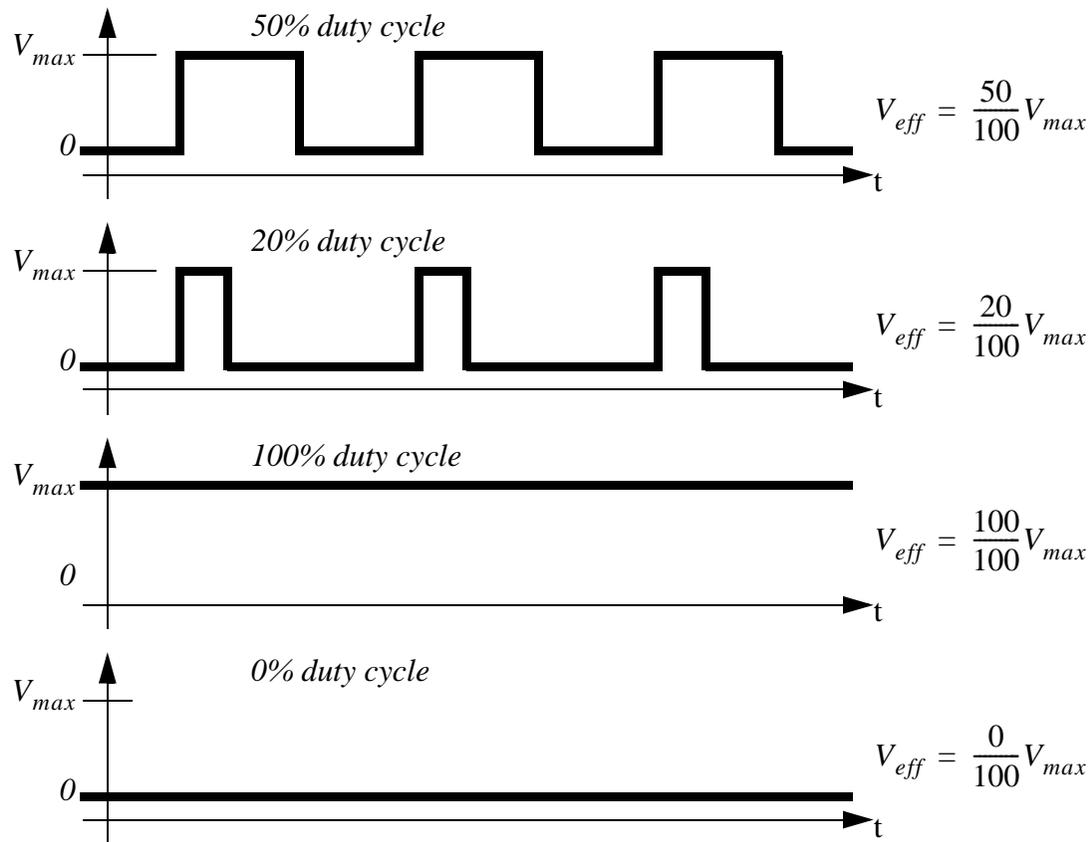
Figure 24.4 Pulse Width Modulation (PWM) For Control
