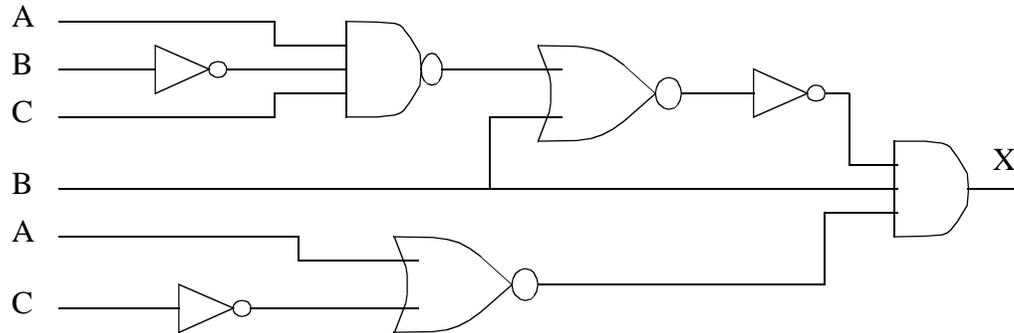
The circuit is converted to a Boolean equation and simplified. The most nested terms in the equation are on the left hand side of the diagram.
