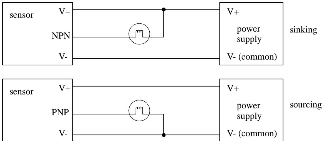
Note: remember to check the current and voltage ratings for the sensors.
