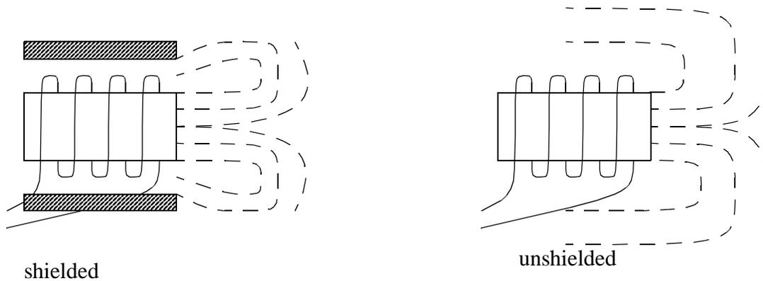
Figure 4.28 Shielded and Unshielded Sensors
