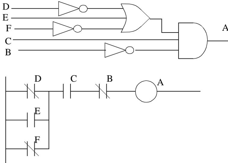
Figure 6.9 The Simplified Form of the Example
