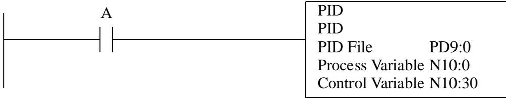
**Description:** This function calculates a value for a control output based on a feedback value. When 'A' is true the instruction will do a PID calculation. In this example the PID calculation is based on the parameters stored in 'PD9:0'. It will use the setpoint 'PD9:0.SP', and the feedback value 'N10:0' to calculate a new control output 'N10:30'. The control variables are normally set using the programming software, although it is possible to set up this instruction using MOV instructions.
