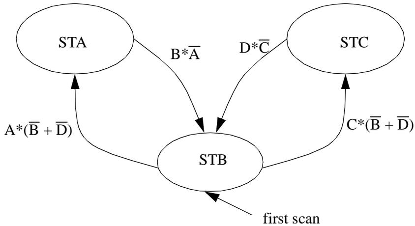
Figure 16.26 A Modified State Diagram to Prevent Racing
