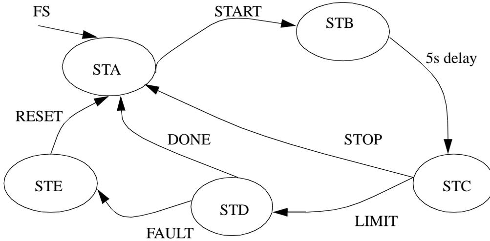
9. The state diagram below is for a simple elevator controller. a) Develop a ladder logic program that implements it with Boolean equations. b) Develop the ladder logic using the block logic technique. c) Develop the ladder logic using the delayed update method.
