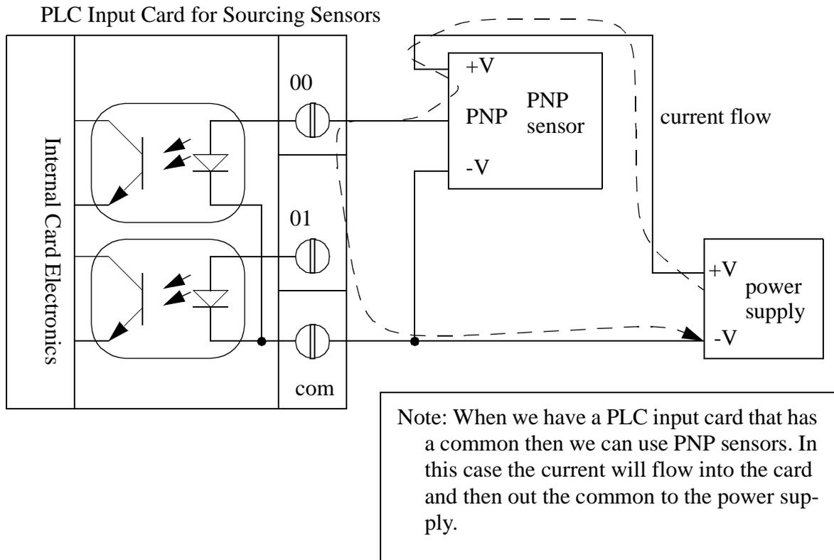
*Figure 4.7* PLC Input Card for Sourcing Sensors
