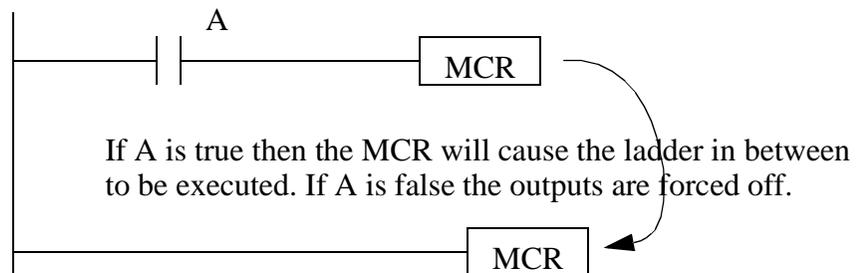
The next section of ladder logic only deals with outputs. For example the output *O/1* is the N/S red light, which will be on for states 1 and 2, or *B3/1* and *B3/2* respectively. Putting normal outputs outside the MCR blocks is important. If they were inside the
