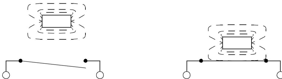
Note: With this device the magnet is moved towards the reed switch. As it gets closer the switch will close. This allows proximity detection without contact, but requires that a separate magnet be attached to a moving part.
