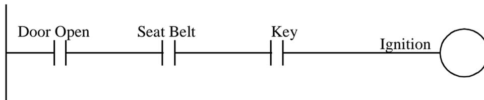
Figure 6.17 Solution to Car Safety System Case
