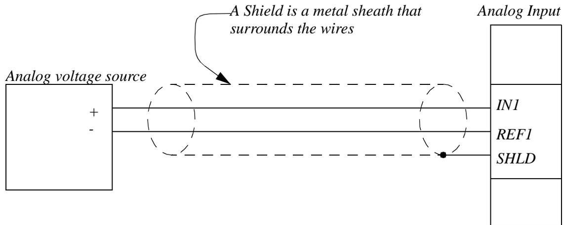
*Figure 23.32* Cable Shielding
