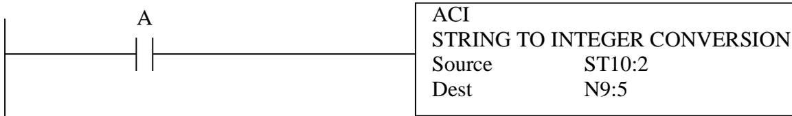
**Description:** The ACI instruction will convert a string to an integer value. In this example it retrieve the string in 'ST10:2', convert it to an integer and store it in 'N9:5'. When converting to an integer it is possible to have an overflow error.
