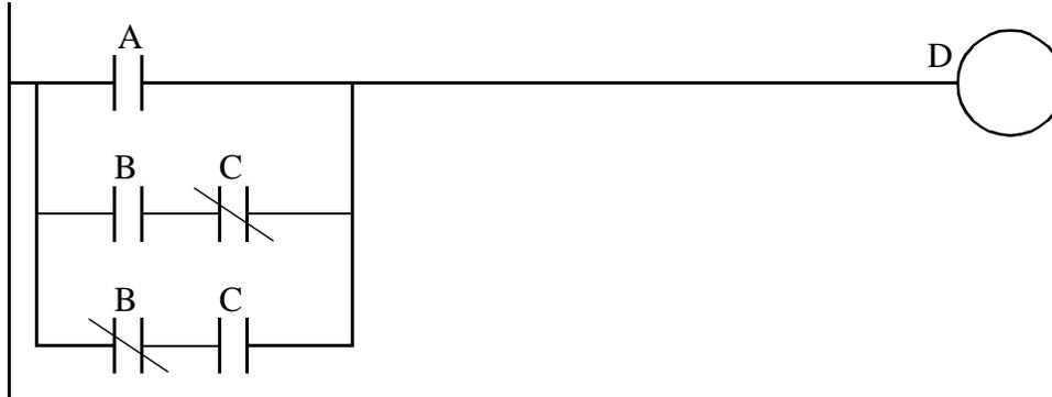
Figure 6.16 Sample Solution for Logic Case Study B
