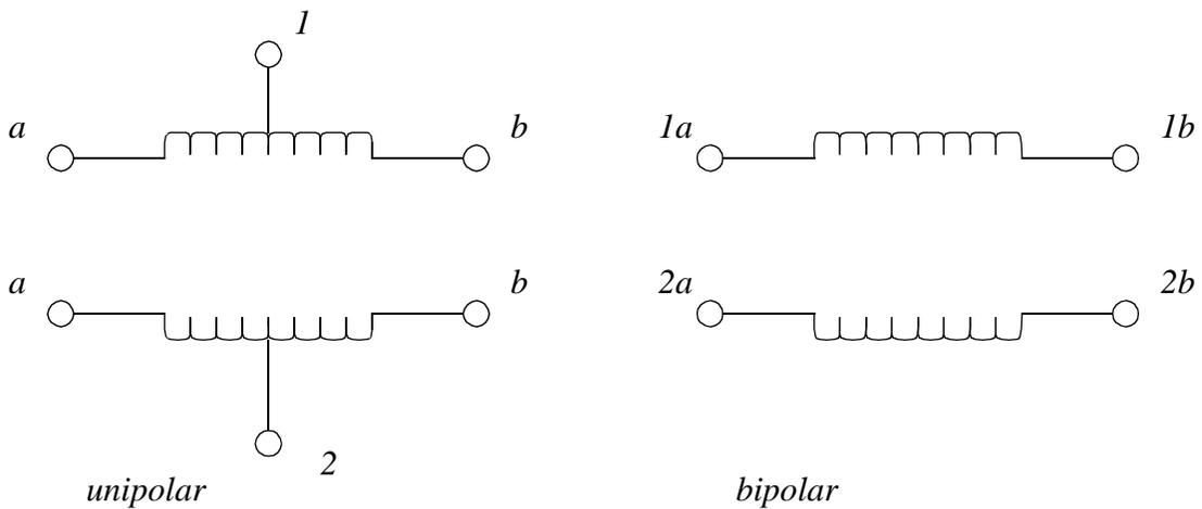
Figure 24.16 Unipolar and Bipolar Stepper Motor Windings
