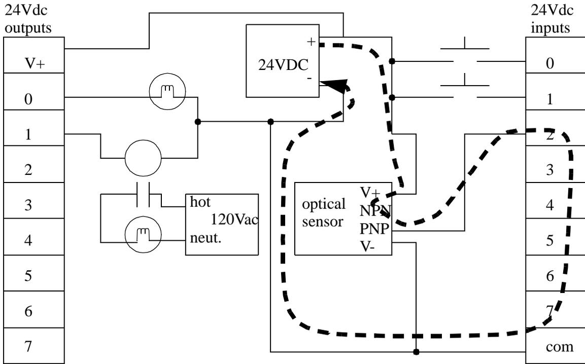
b) the PNP output was selected. because it will supply current, while the input card requires it. The dashed line indicates the current flow through the sensor and input card.
