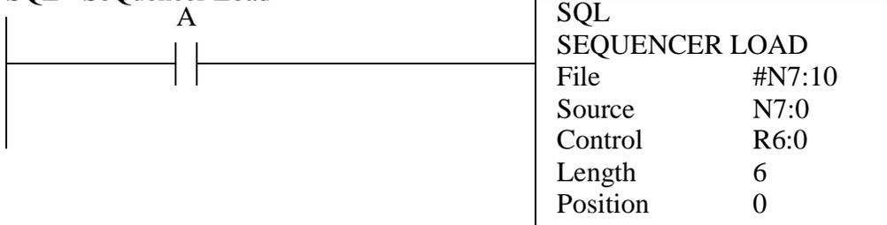
**Description:** When the input goes from false to true the value at the source will be loaded into the sequencer. After the position has reached the length the following values will be ignored, and the done bit will be set.
