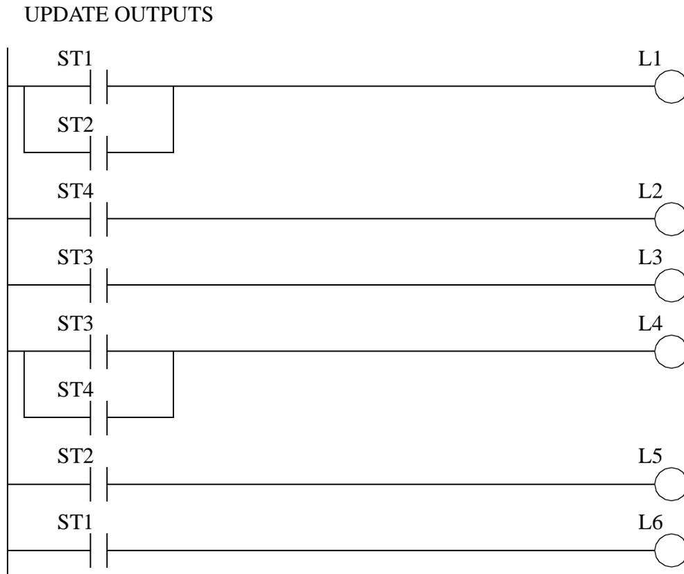
*Figure 12.30* Ladder Logic for the State-Transition Equations
