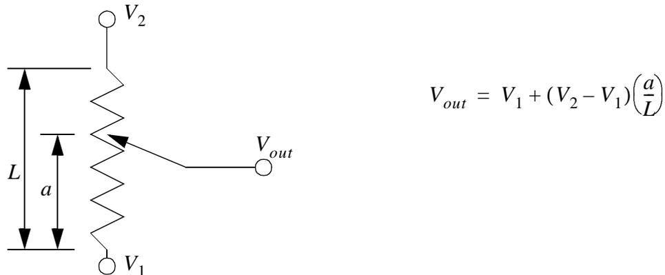
Figure 23.7 Linear Potentiometer
