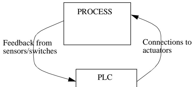
Figure 2.9 The Separation of Controller and Process
