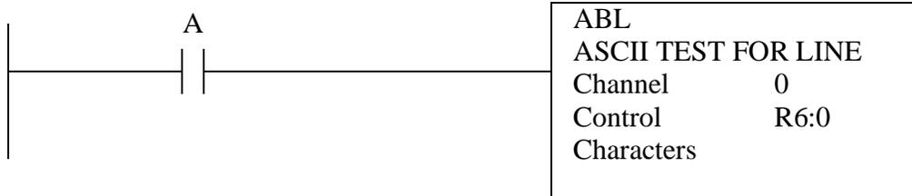
**Description:** The ABL instruction checks for available characters in the input buffer. In this example, when 'A' goes true the function will check the input buffer for channel '0' and put characters in 'R6:0.POS'. The count will include end of line characters such as 'CR' and 'LF'. The ACB instruction is the same, except that it does not include the end of line characters.
