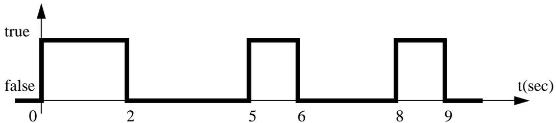
2. Design ladder logic for the timing diagram below. When an input *A* becomes active the sequence should start.
