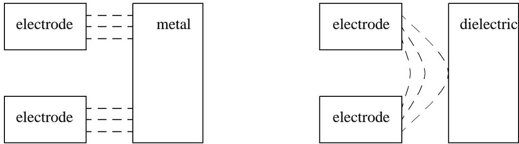
*Figure 4.24* Dielectrics and Metals Increase the Capacitance
