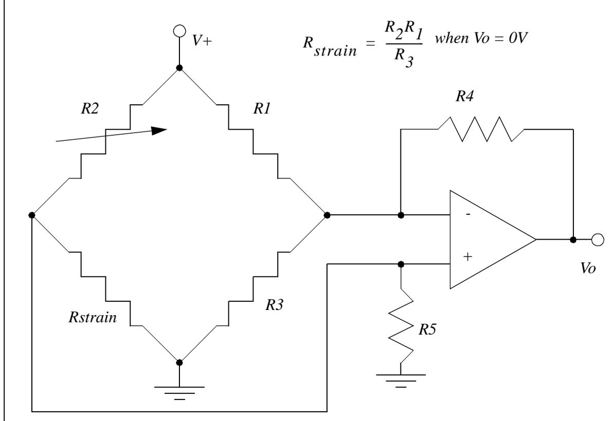
*Figure 23.18* Measuring Strain with a Wheatstone Bridge
