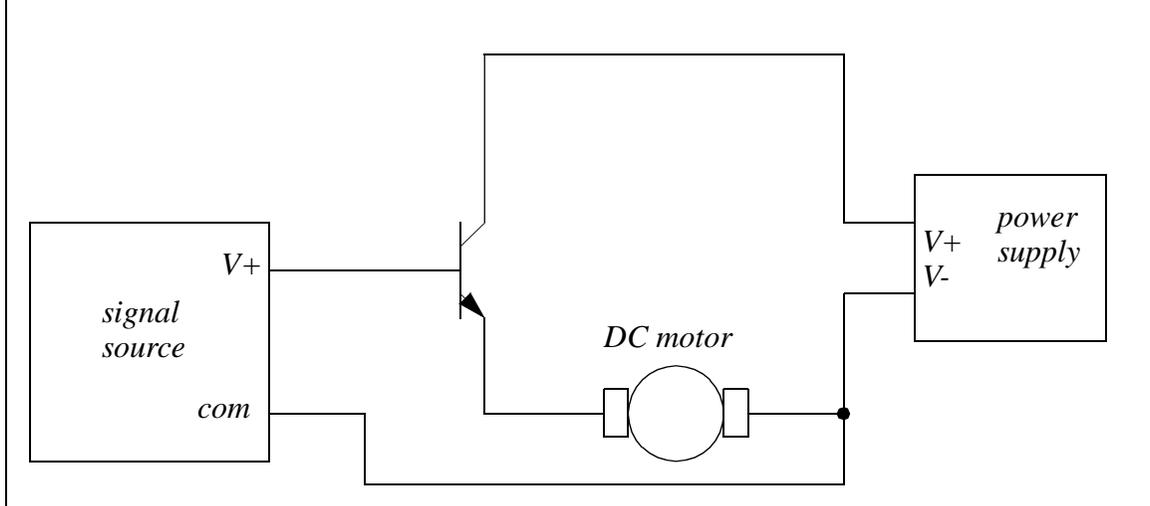
Figure 24.5 PWM Unidirectional Motor Control Circuit
