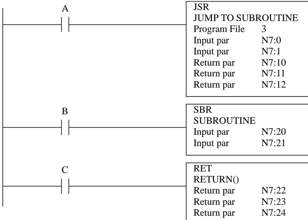
**Description:** The JSR will jump to another program file and pass a list of arguments that can be a variable length. The first statement in the subroutine program file should be SBR to retrieve the arguments passed. The subroutine will end with the RET command that will go back to where the JSR function was encountered. The RET function can return a variable number of arguments.
