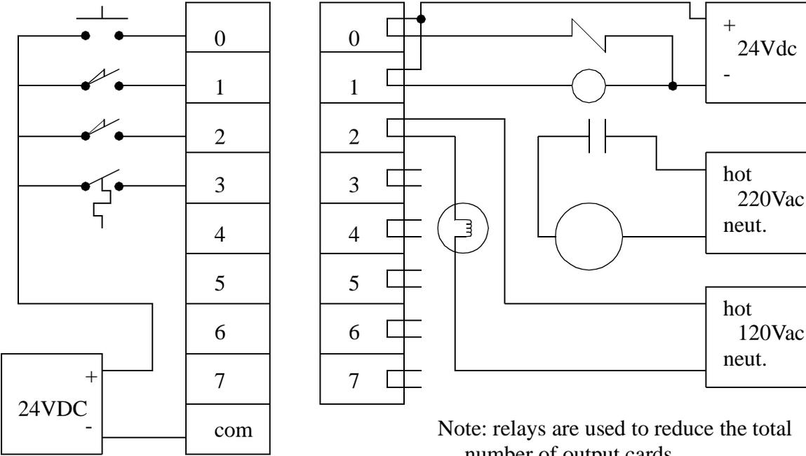
Note: relays are used to reduce the total number of output cards
