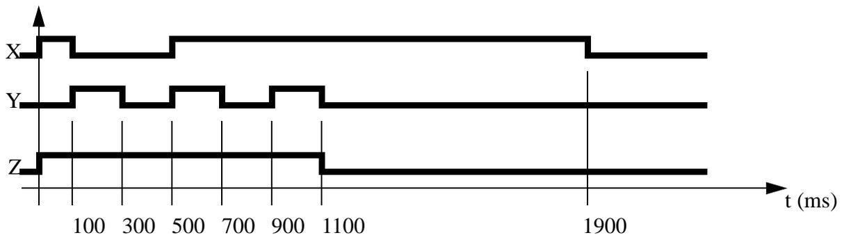
3. A wrapping process is to be controlled with a PLC. The general sequence of operations is described below. Develop the ladder logic using process sequence bits.
