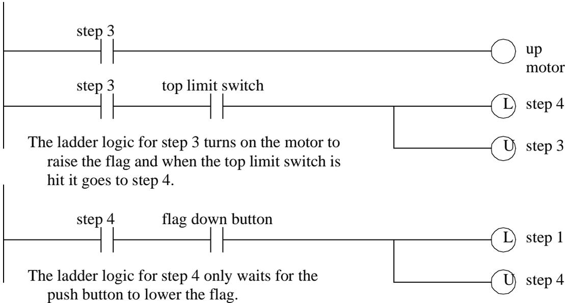
Figure 10.3 A Process Sequence Bit Design Example (continued)
