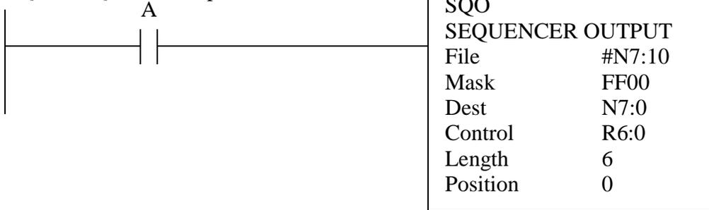
**Description:** When the input goes from false to true the sequencer will output a value from a new position in the sequencer table. After the position has reached the length the sequencer will reset to position 1. Note that the first entry in the sequencer table will only be output the first time the function is un, or if reset has been used.
