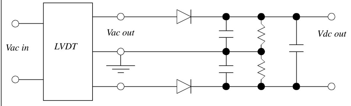
Figure 23.9 A Simple Signal Conditioner for an LVDT
