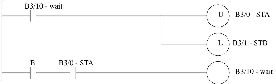
Figure 16.27 Subroutines for State STA to Prevent Racing
