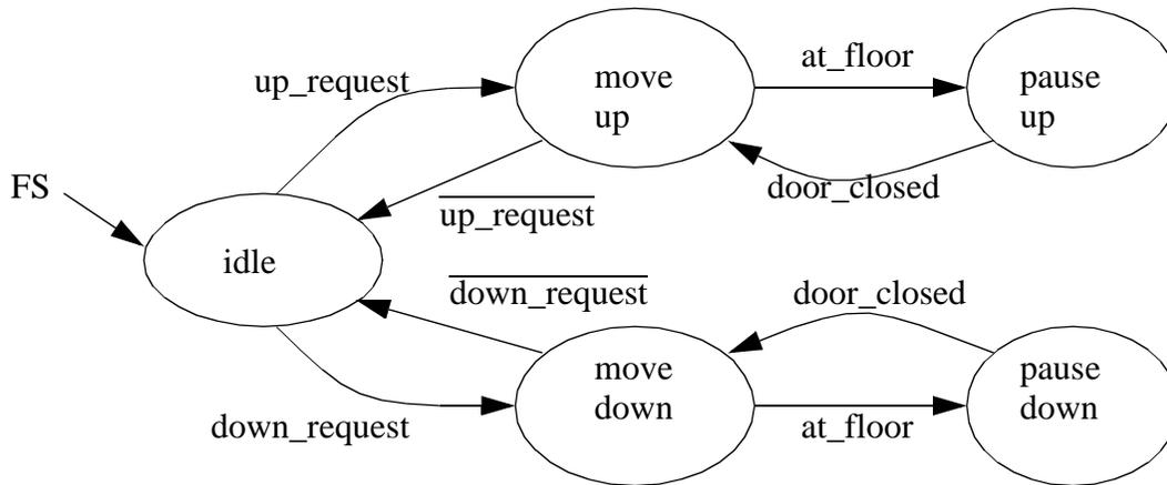
10. Write ladder logic for the state diagram below a) using an equation based method. b) without
