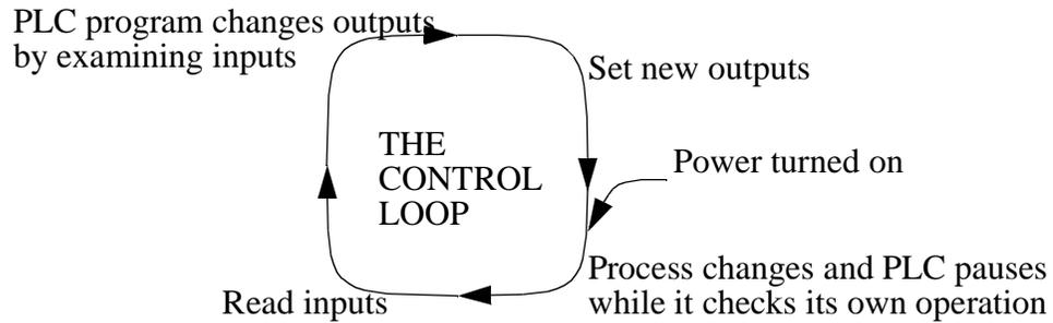
Figure 2.10 The Scan Cycle of a PLC
