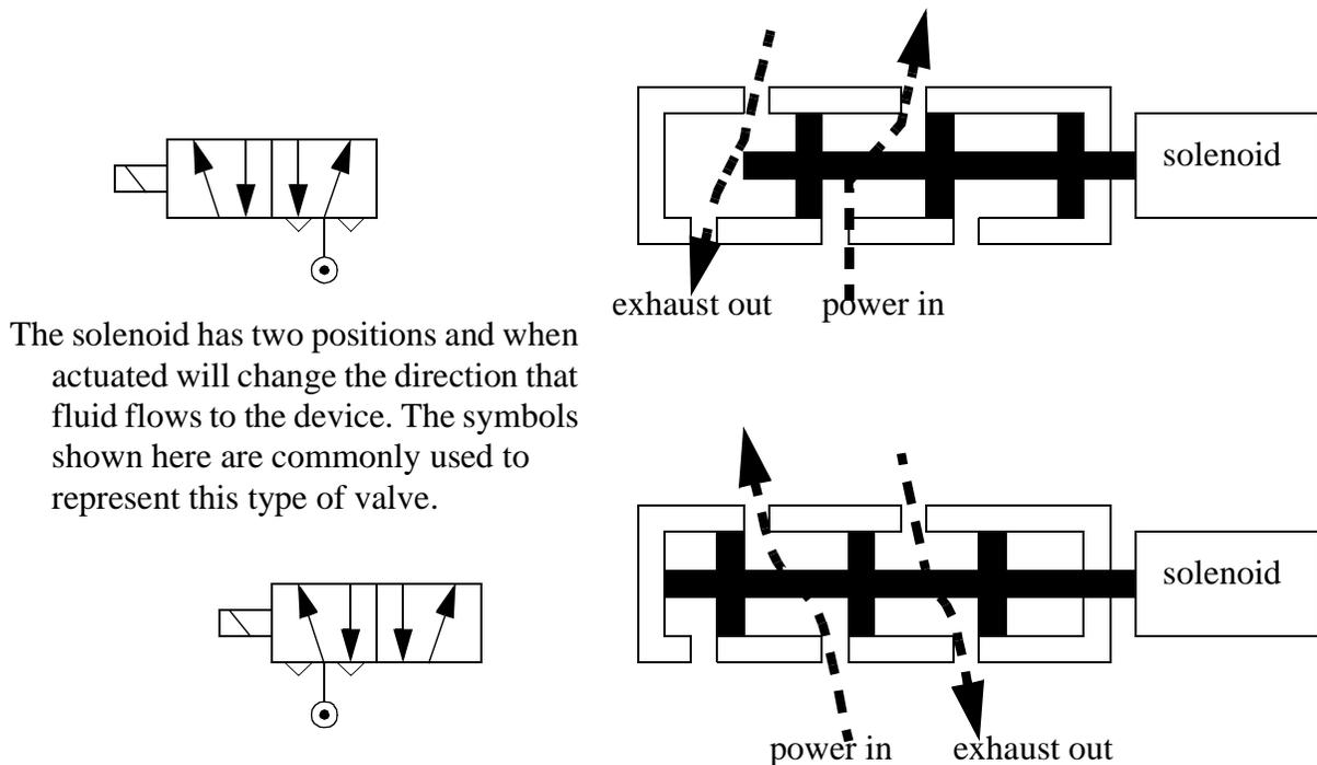
Figure 5.2 A Solenoid Controlled 5 Ported, 4 Way 2 Position Valve
