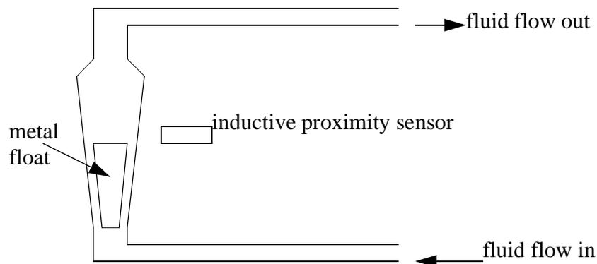
As the fluid flow increases the float is forced higher. A proximity sensor can be used to detect when the float reaches a certain height.
