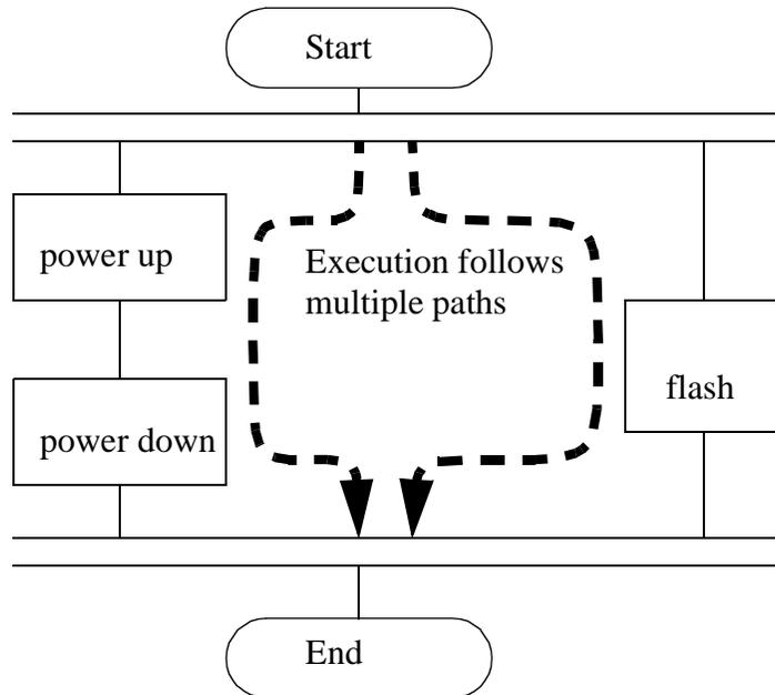
Figure 2.7 An Example of a Sequential Function Chart
