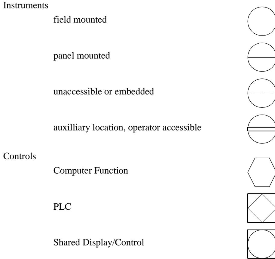
Figure 32.2 Symbols for Functions and Instruments
