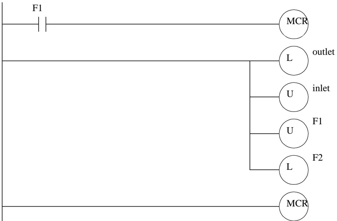
Figure 11.6 Ladder Logic for the Operation *F1*
