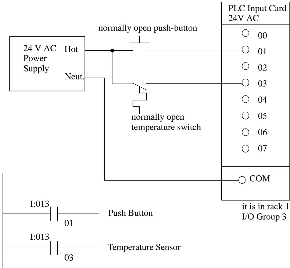
Figure 3.2 An AC Input Card and Ladder Logic
