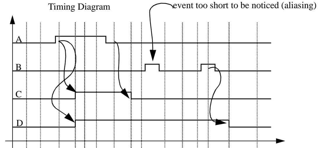
These lines indicate PLC input/output refresh times. At this time all of the outputs are updated, and all of the inputs are read. Notice that some inputs can be ignored if at the wrong time, and there can be a delay between a change in input, and a change in output.
