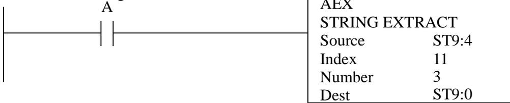
**Description:** This function will remove part of a string. In this example the characters in the 12th, 13th and 14th positions ('3' charaters starting at the 11th position), are copied to the location ST9:0. The original string is not changed.
