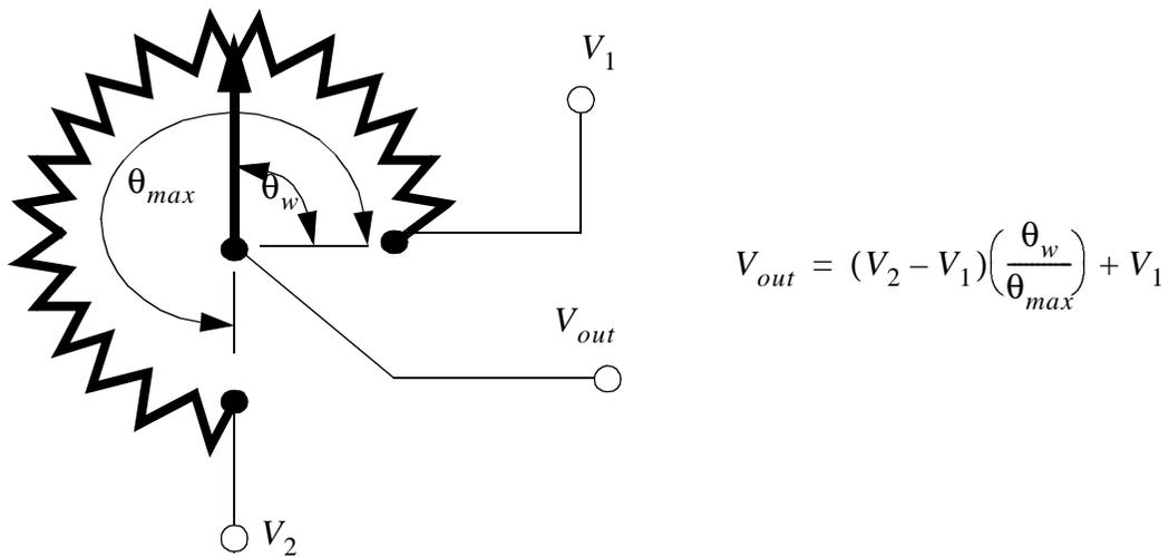
Figure 23.2 A Potentiometer as a Voltage Divider
