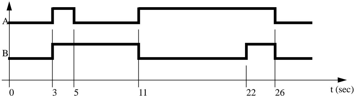
3. Use the timing diagram below to design ladder logic. The sequence should start when input *X* turns on. *X* may only be on momentarily, but the sequence should execute anyway.
