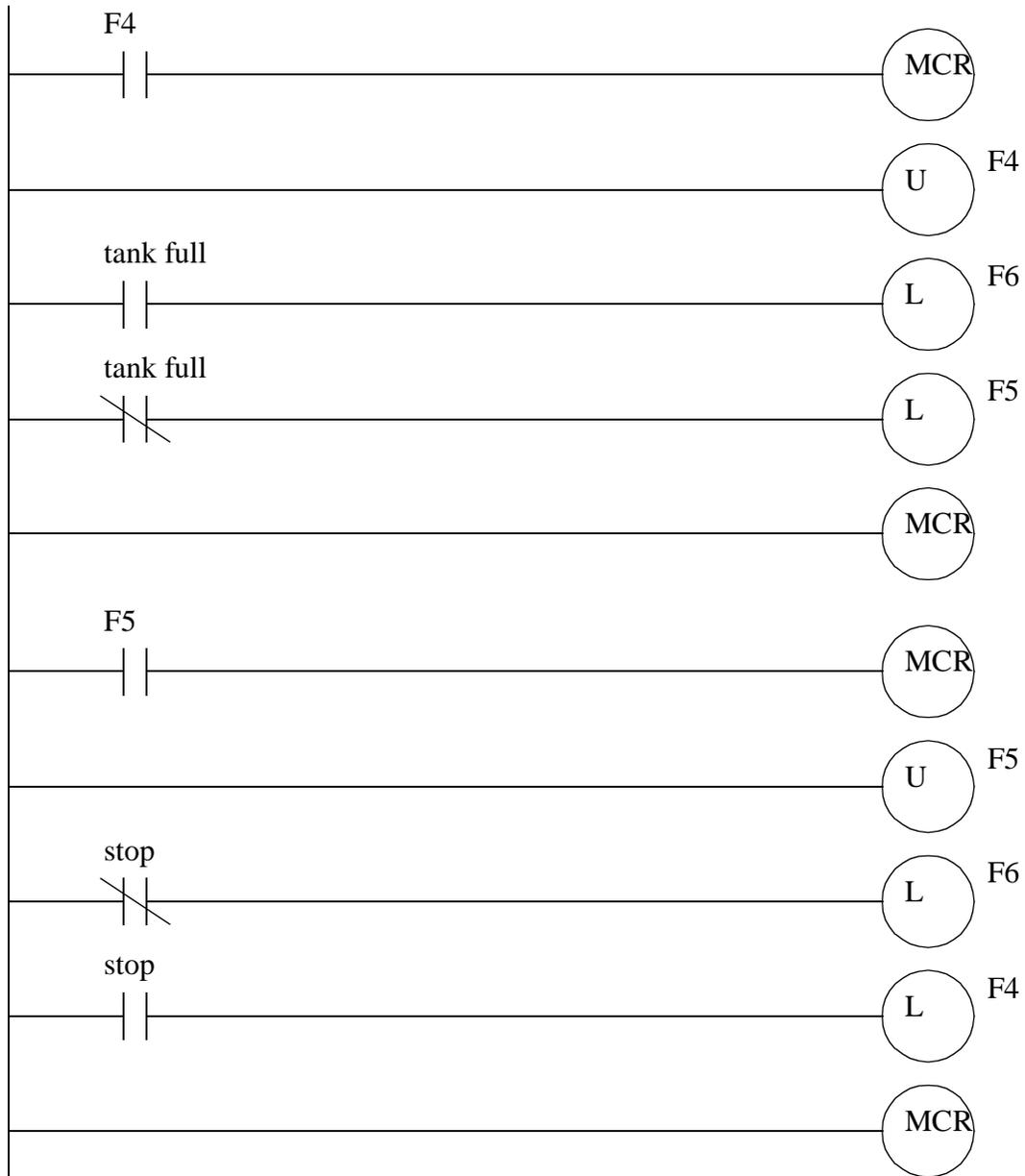
Figure 11.8 Ladder Logic for Operations *F4* and *F5*
