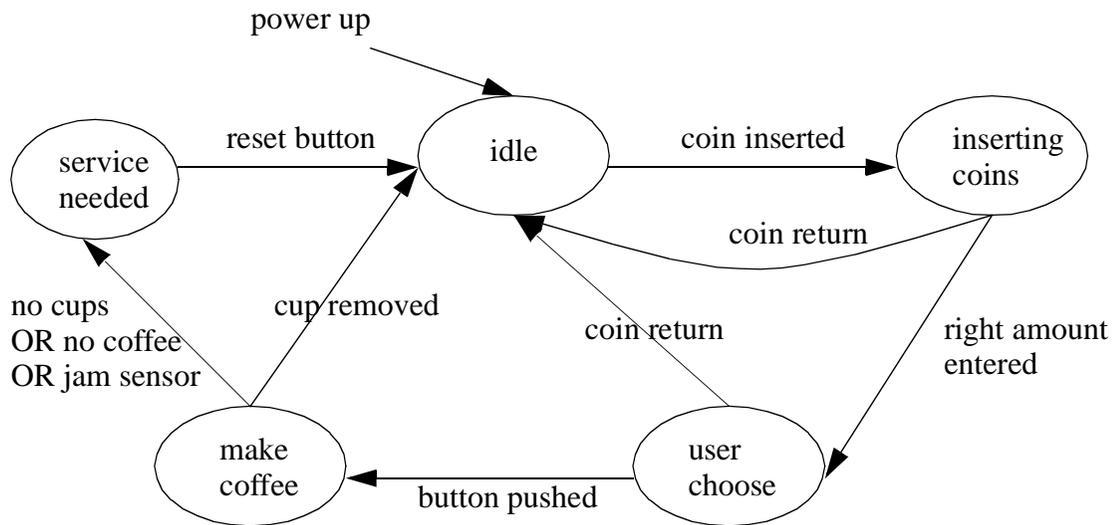
Figure 12.3 State Diagram for a Coffee Machine
