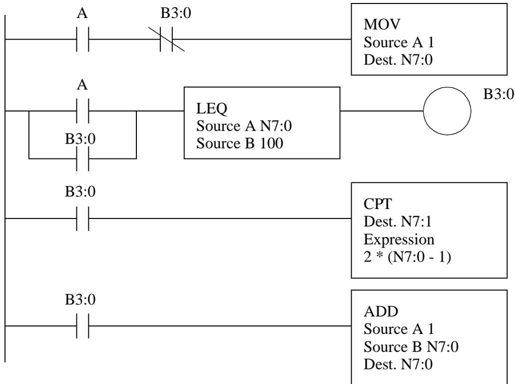
Figure 15.26 A Series Calculation Example
