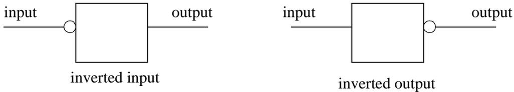
Figure 21.2 Inverting Inputs and Outputs on Function Blocks
