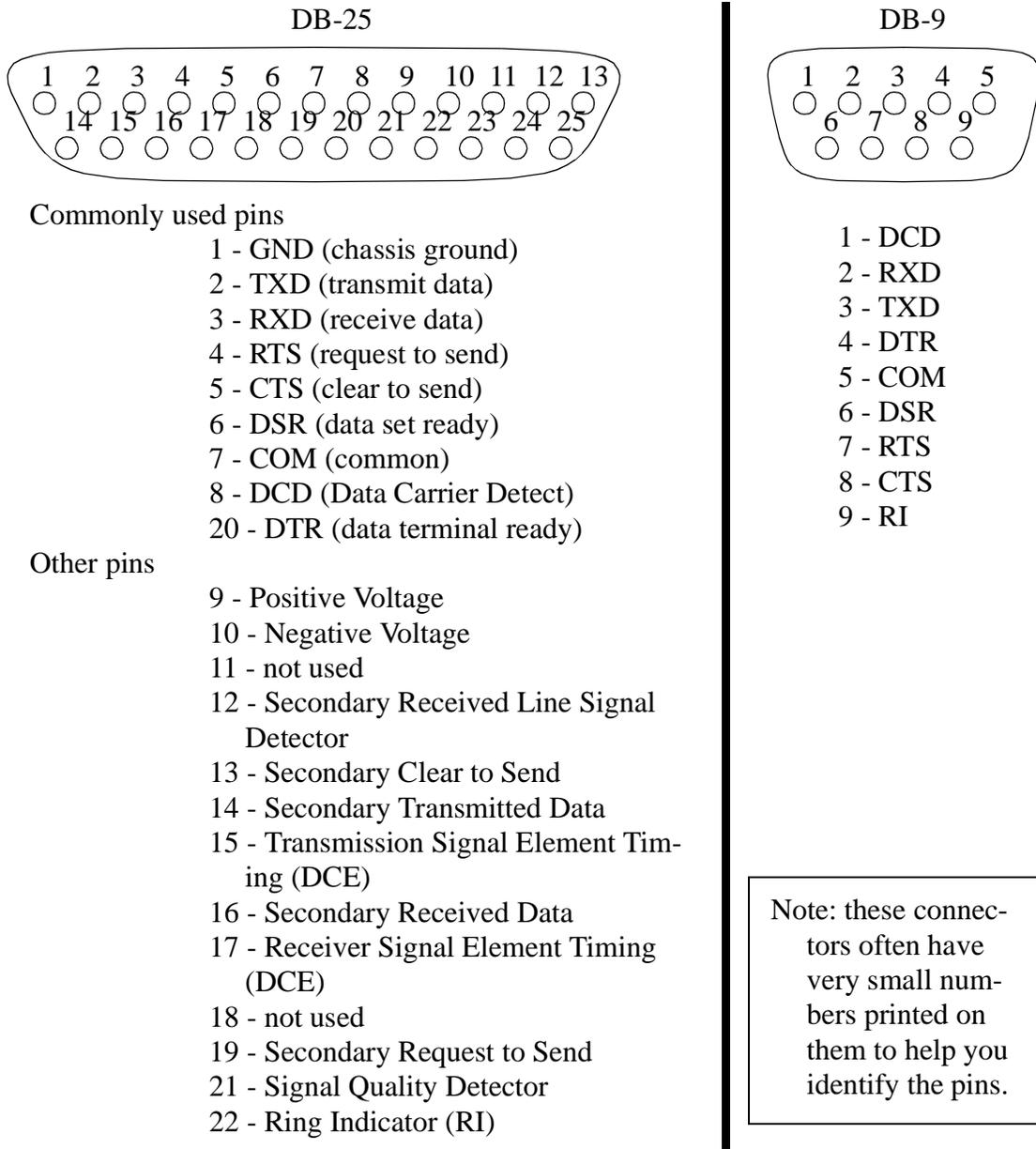
Figure 27.5 Typical RS-232 Pin Assignments and Names
