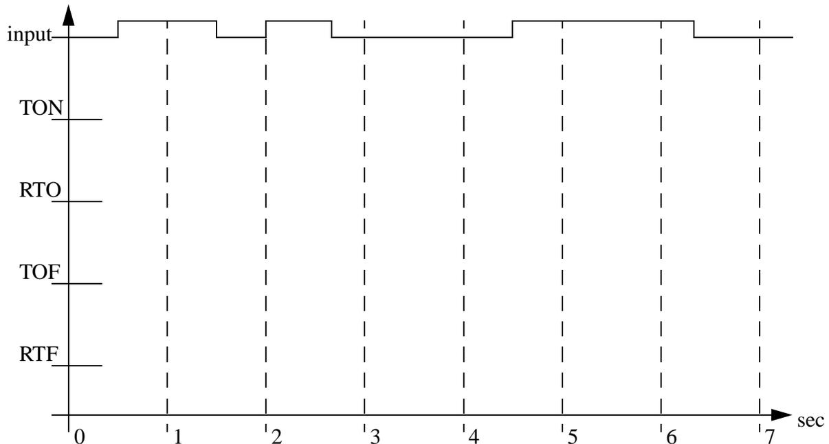
10. Design ladder logic that allows an RTO to behave like a TON.
