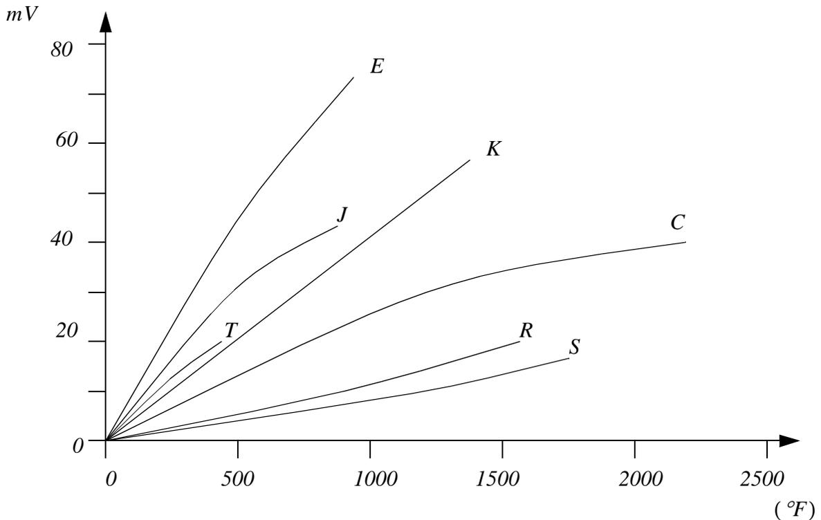
Figure 23.28 Thermocouple Temperature Voltage Relationships (Approximate)
