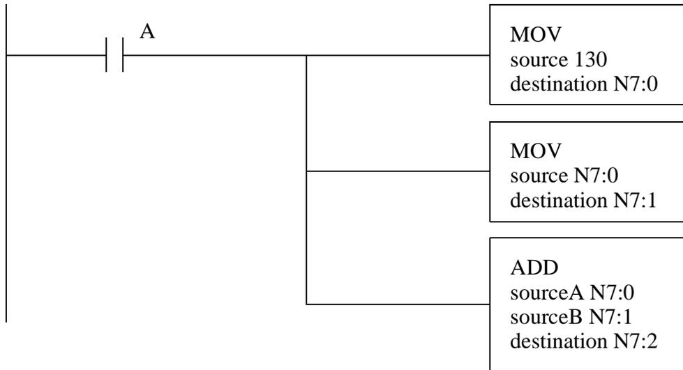
Figure 14.11 An Example of Ladder Logic Functions
