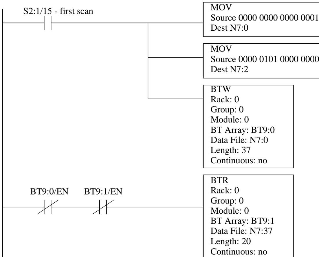
Figure 25.11 Implementing a Proportional Controller with Ladder Logic
