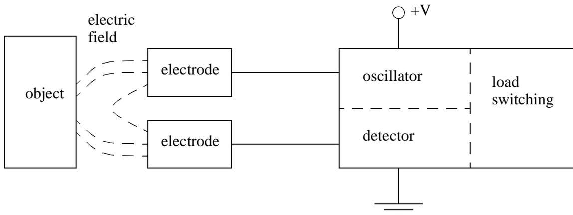
NOTE: For this sensor the proximity of any material near the electrodes will increase the capacitance. This will vary the magnitude of the oscillating signal and the detector will decide when this is great enough to determine proximity.
