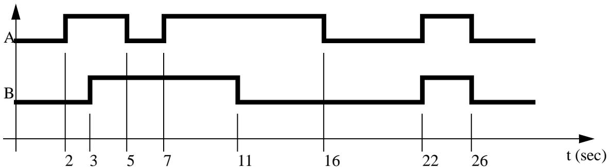
4. Write a program that will execute the following steps. When in steps b) or d), output *C* will be true. Output *X* will be true when in step c).
