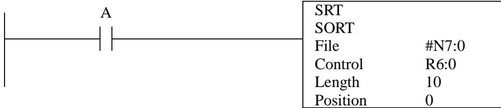
**Description:** This functions sort the values in memory from lowest value in the first location to the highest value. When the input goes from false to true the calculation is begun. The values to be used for the calculation are sorted in the memory starting at the start of the file location, for the length indicated. The control file is used for the calculation to keep track of position, and indicate when the calculation is done (it may take more than one PLC scan).
