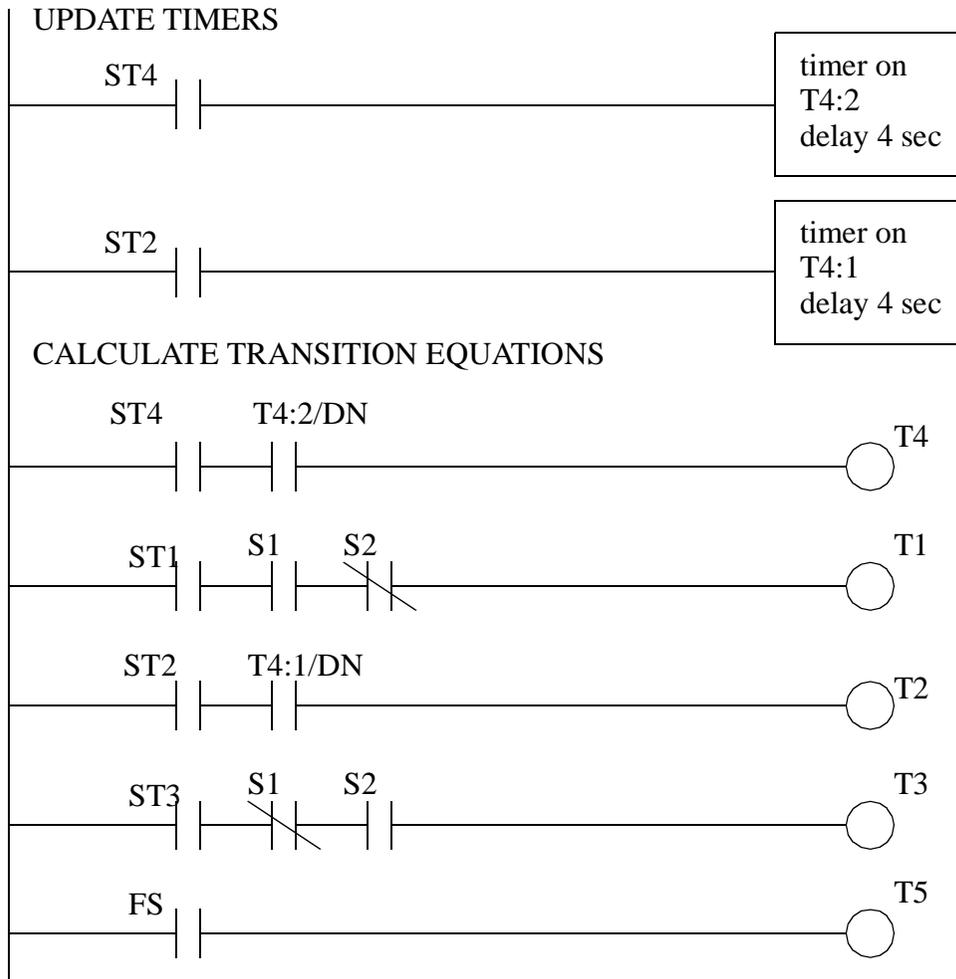
Figure 12.28 Ladder Logic for the State-Transition Equations
