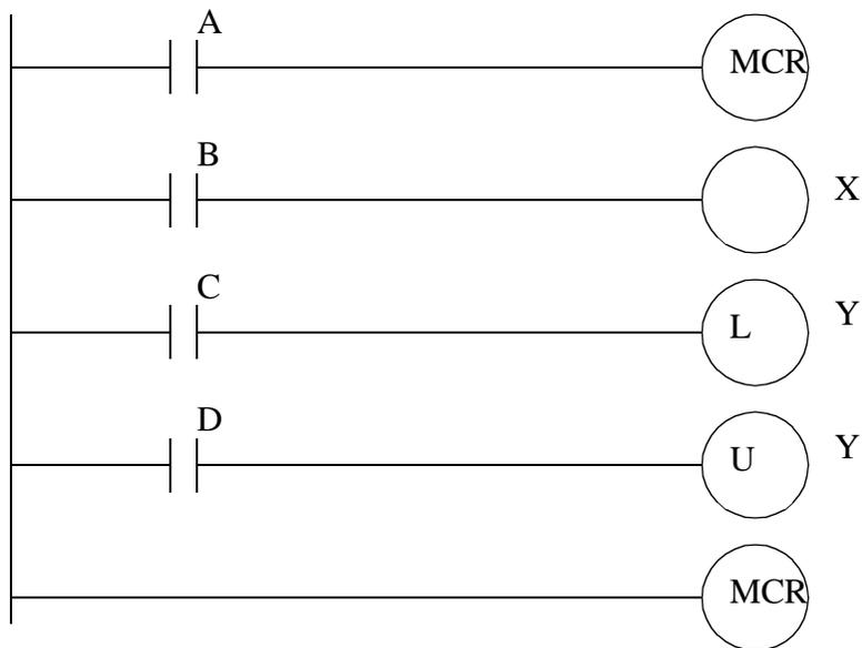
Note: If a normal input is used inside an MCR block it will be forced off. If the output is also used in other MCR blocks the last one will be forced off. The MCR is designed to fully stop an entire section of ladder logic, and is best used this way in ladder logic designs.
