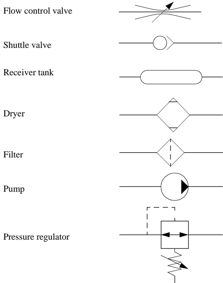
*Figure 5.7* Pneumatics Components
