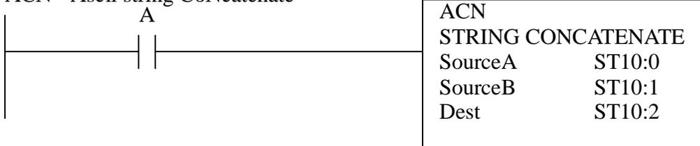
**Description:** This will concatenate two strings together into one combined string. In this example while 'A' is true the strings in 'ST10:0' and 'ST10:1' will be added together and stored in 'ST10:2'.
