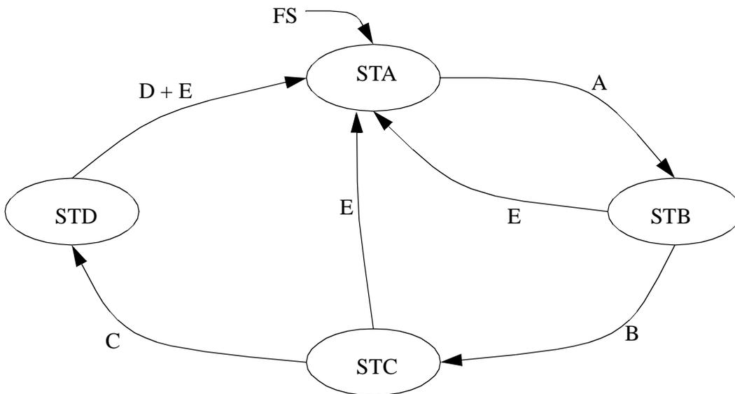
6. Implement the State-Transition equations.in the figure below with ladder logic.
