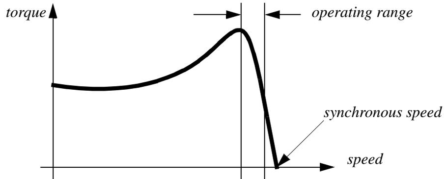
Figure 24.10 Torque Speed Curve for an Induction Motor
