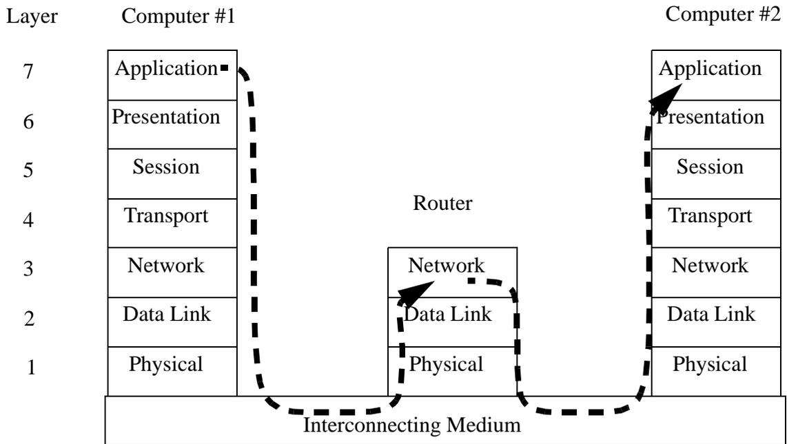
Figure 28.5 The OSI Network Model with a Router
