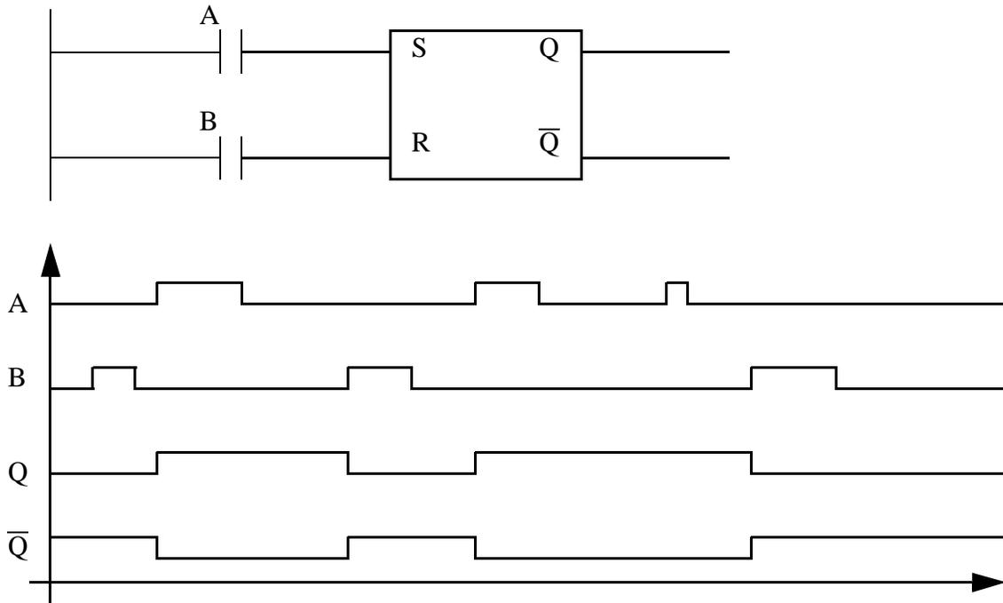
Figure 9.6 Flip-Flops for Latching Values
