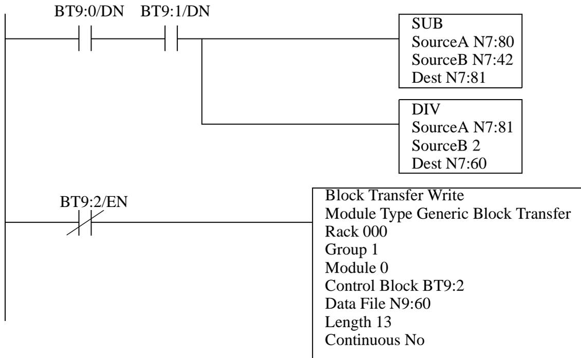
Figure 25.21 A Water Tank Level Control Program
