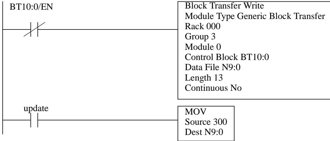
Figure 22.13 Controlling a 1771-OFE Analog Output Card
