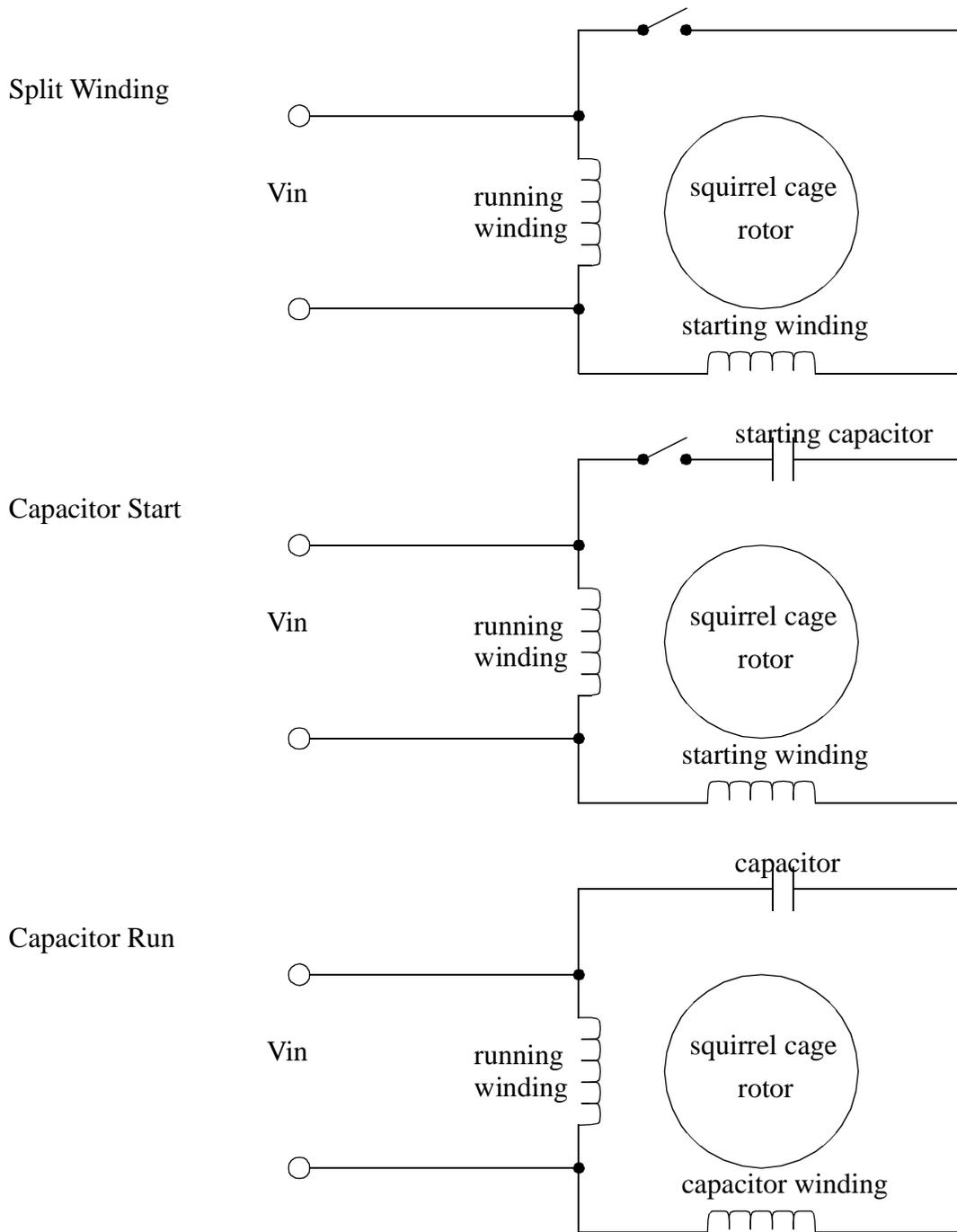
Figure 24.12 Single Phase Motor Configurations
