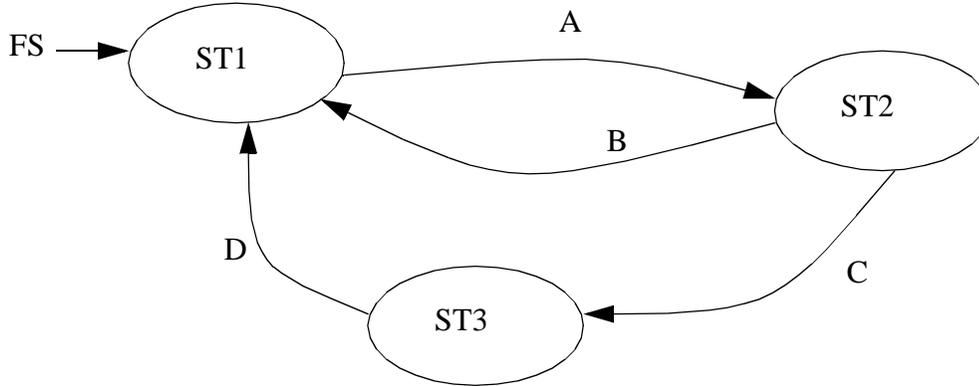
3. Convert the following state diagram to ladder logic using the block logic method. Give the stop button higher priority.
