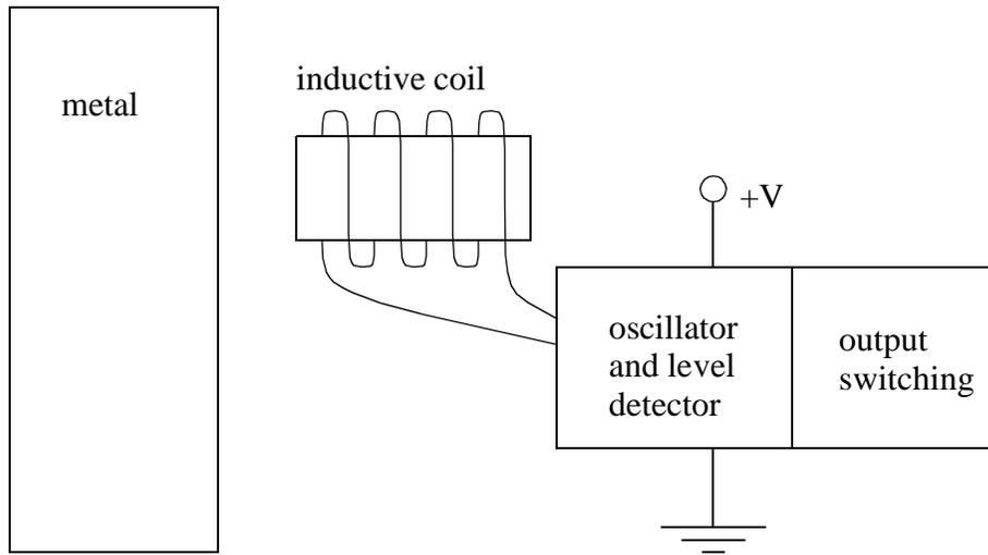
Note: these work by setting up a high frequency field. If a target nears the field will induce eddy currents. These currents consume power because of resistance, so energy in the field is lost, and the signal amplitude decreases. The detector examines field magnitude to determine when it has decreased enough to switch.
