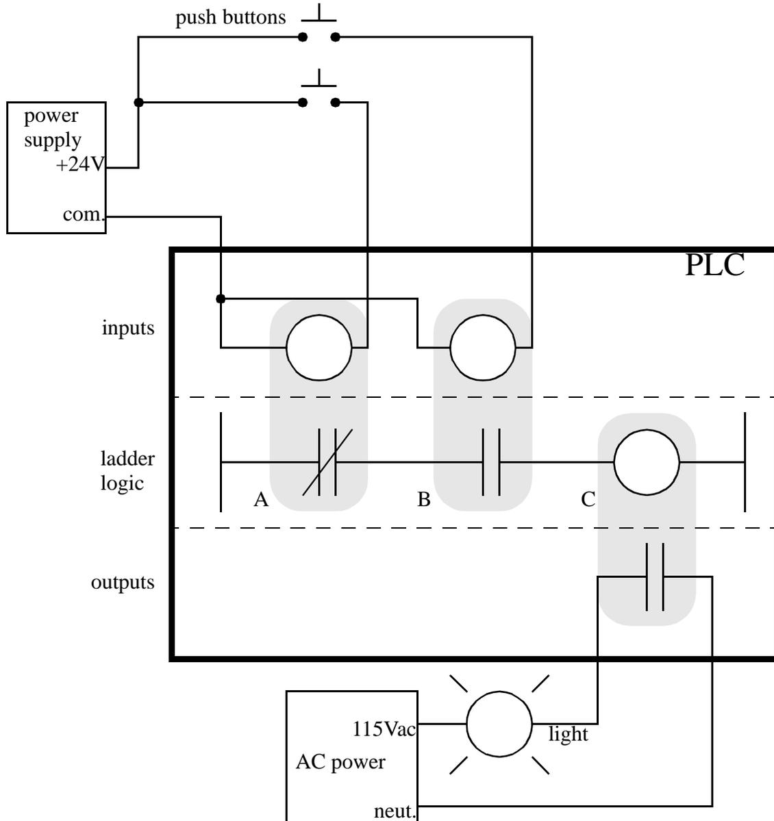
Figure 2.3 A PLC Illustrated With Relays
