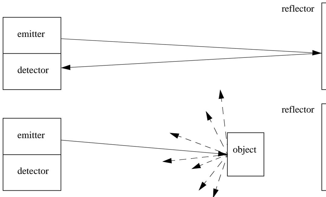
Note: the reflector is constructed with polarizing screens oriented at 90 deg. angles. If the light is reflected back directly the light does not pass through the screen in front of the detector. The reflector is designed to rotate the phase of the light by 90 deg., so it will now pass through the screen in front of the detector.
