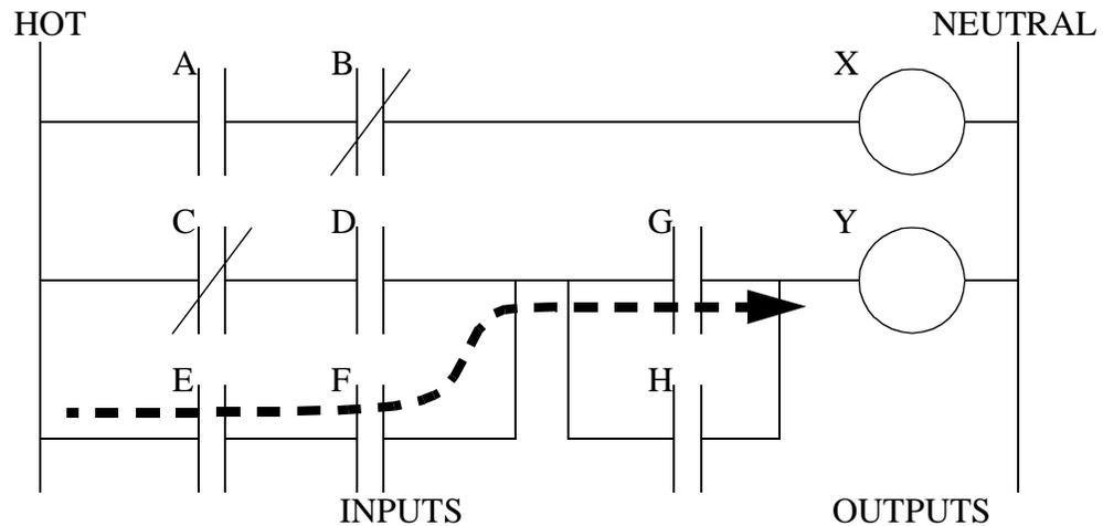
Note: Power needs to flow through some combination of the inputs (A,B,C,D,E,F,G,H) to turn on outputs (X,Y).
